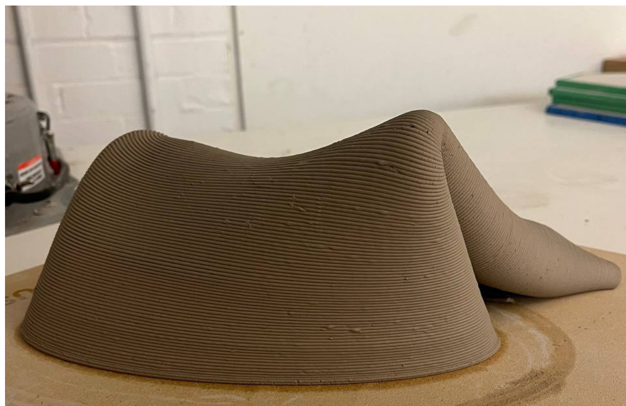
Figure 4.43. The collapse of primary twisted pieces due to the material' weight. The piece collapsed during the printing process due to the unbalanced weight distribution.
