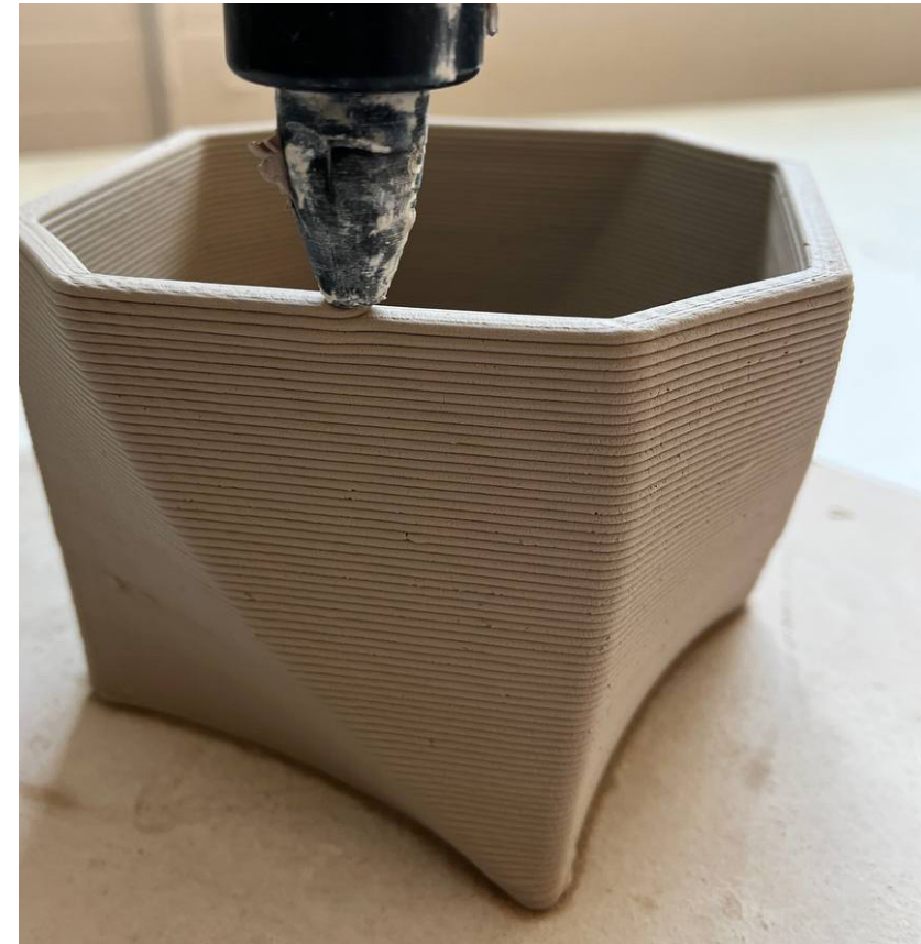
Figure 4.46. Right. The second middle brick with faces curved outward.
