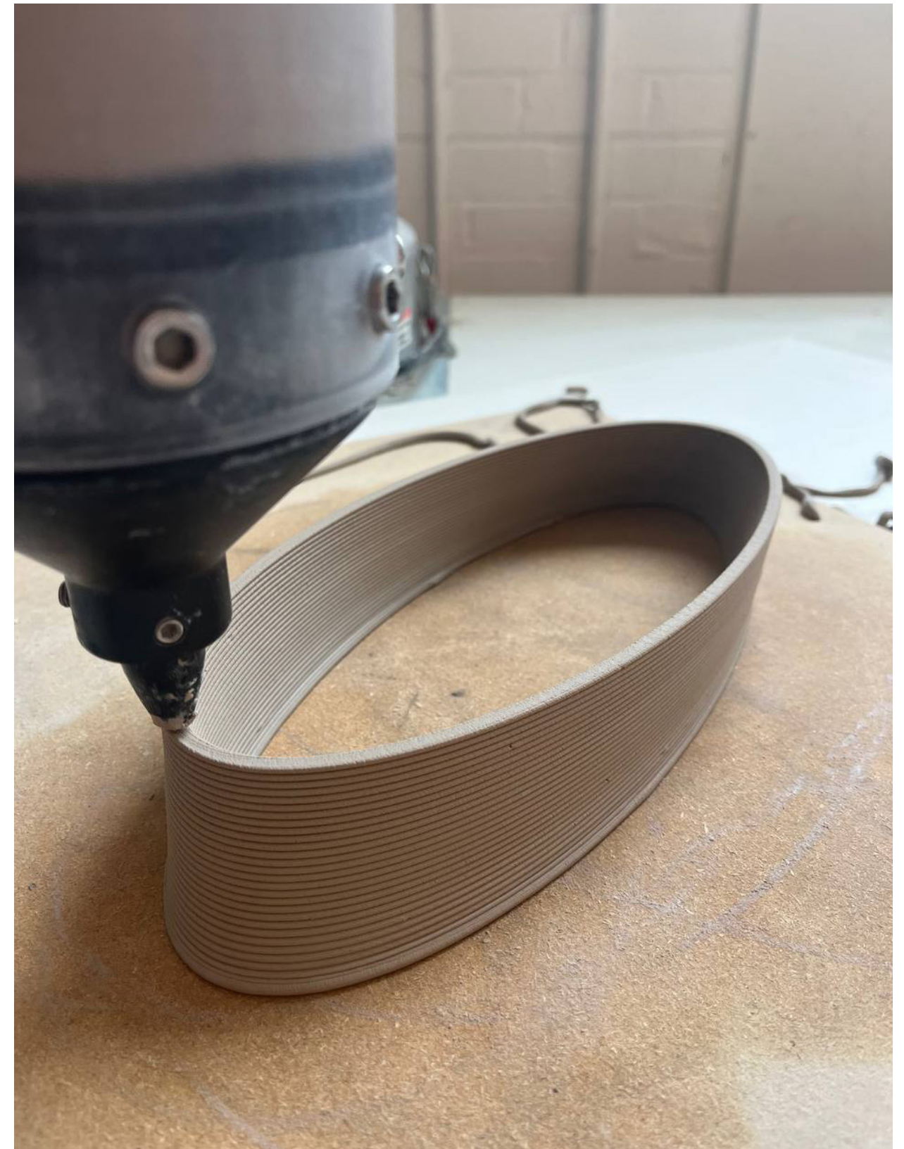
Figure 4.44. The twisted geometry of the bricks for screen 2. The bottom part of the ellipses might need to be hardened, using the heat gun.
