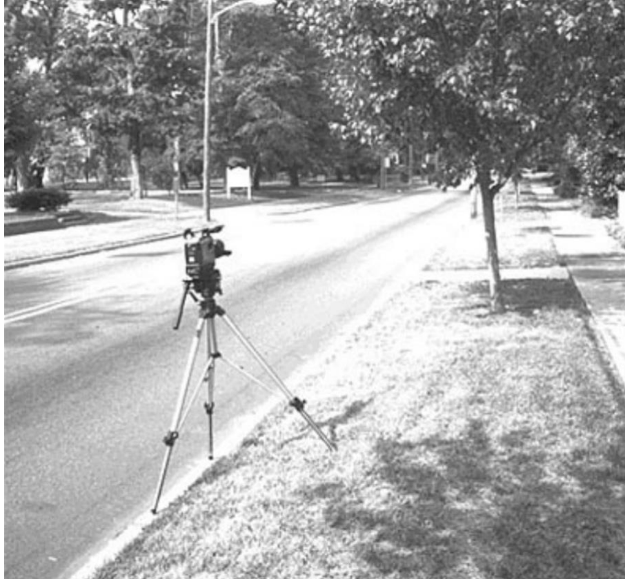
Figure 2: Camera Position for Videoclip Recording for BCI (FHWA, 1998)
