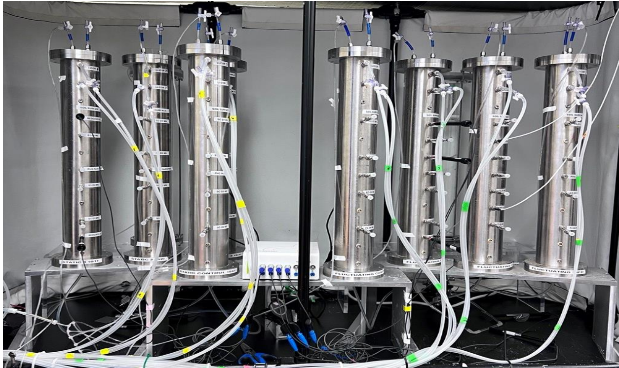
Figure 3-1: A photo of the stainless-steel columns equipped with moisture, temperature, and redox sensors, and water and gas samplers.
