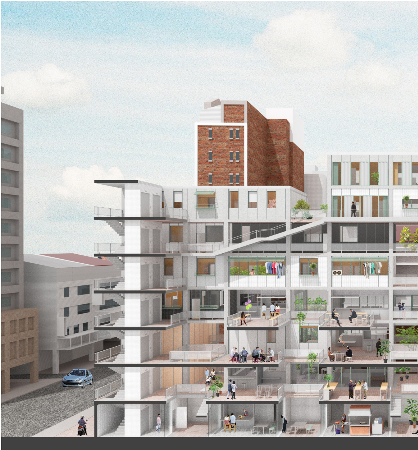
Fig. 5.140 The internal courtyard expresses the different combinations of window types, finishes, and facade additions used by businesses and households to customize their units.
