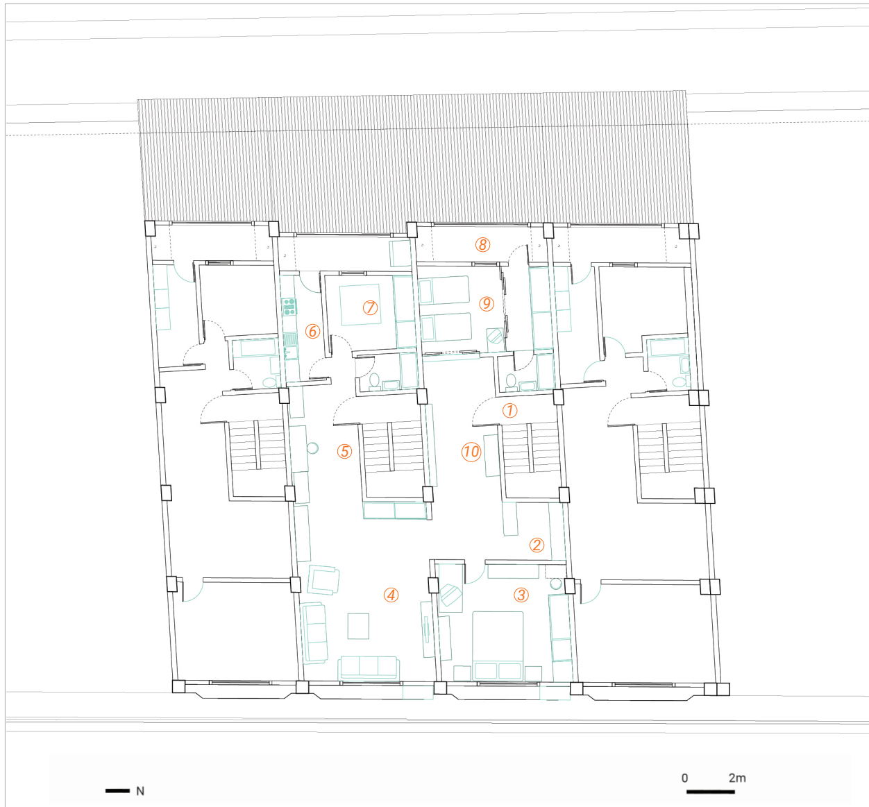
Fig. 4.70 The fifth level of the streethouse showing how two units are combined through the removal of a partition wall.
