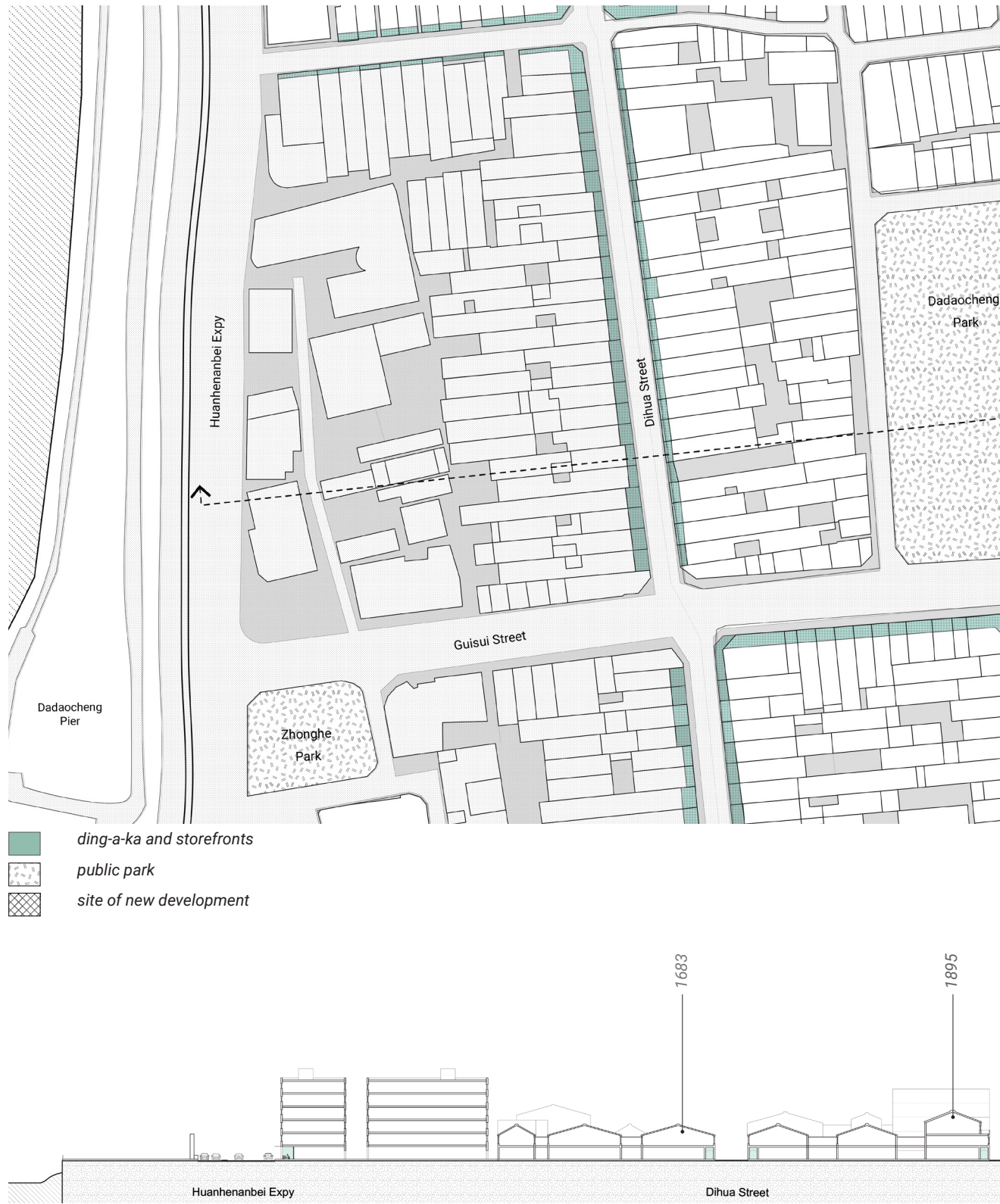
Fig. 3.58 Site context and section highlighting the continuous urban corridor formed collectively by the ding-a-ka's of the streethouses.
