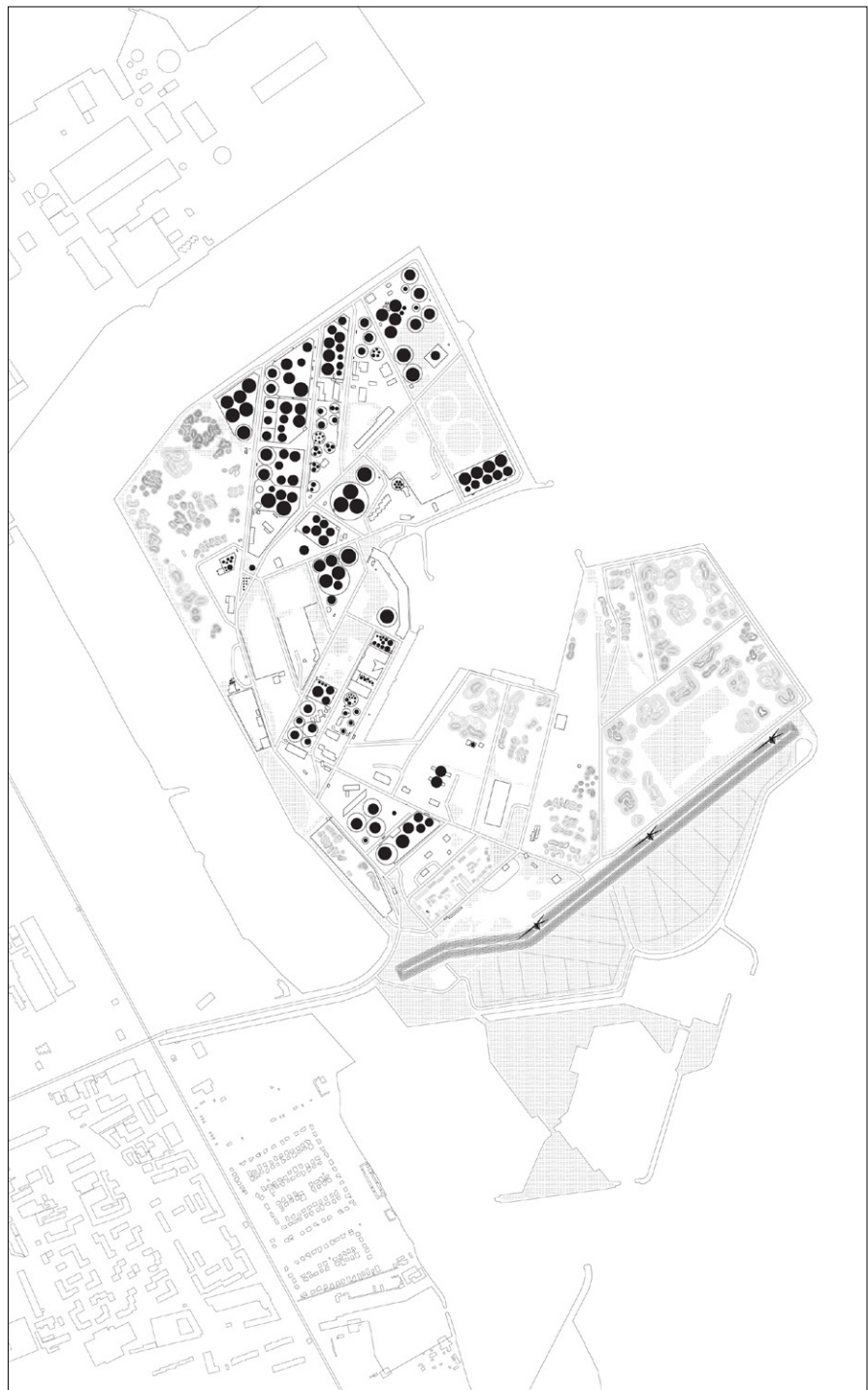
Fig. 4.1 Plan drawing of existing conditions on Petrol Island. Black fill indicates oil tanks remaining. Drawing by author.
