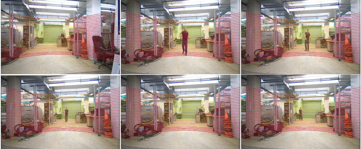
Figure 3.4: Illustration of several frames showing the projected LIDAR point cloud on the image captured. Despite the object moving to different extents of the image, the projection remains accurate.
