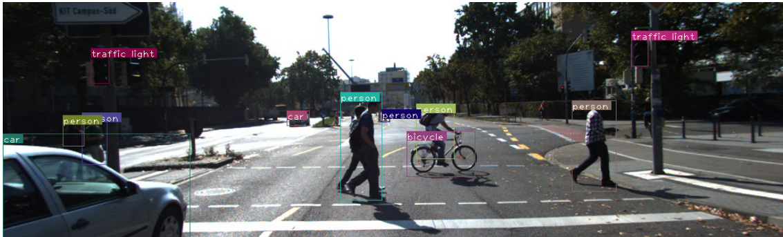
Figure A.3: Classified output detections and bounding boxes from Yolo4.
