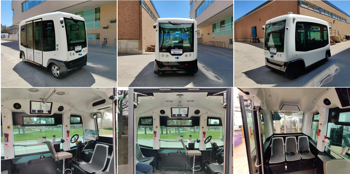
Figure 6.1: Illustration of the WATonoBus platform equipped with cameras, LIDARs, GPS, computing, and an autonomous software stack used to perform experiments.
