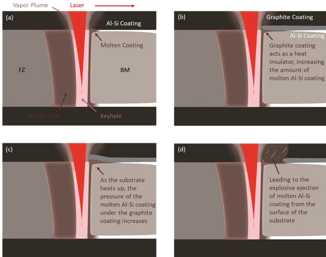
Figure 49: Schematic showing the mechanism of removal of Al-Si coating during the laser welding of graphite coated 22MnB5 steel where (a) is the welding process with no graphite coating, (b) is the process with the graphite coating showing an increase in the amount of molten Al-Si coated sandwiched between the graphite coating and the substrate, and (c and d) is showing how the molten Al-Si coating becomes pressurized and explodes through the graphite coating, respectively.
