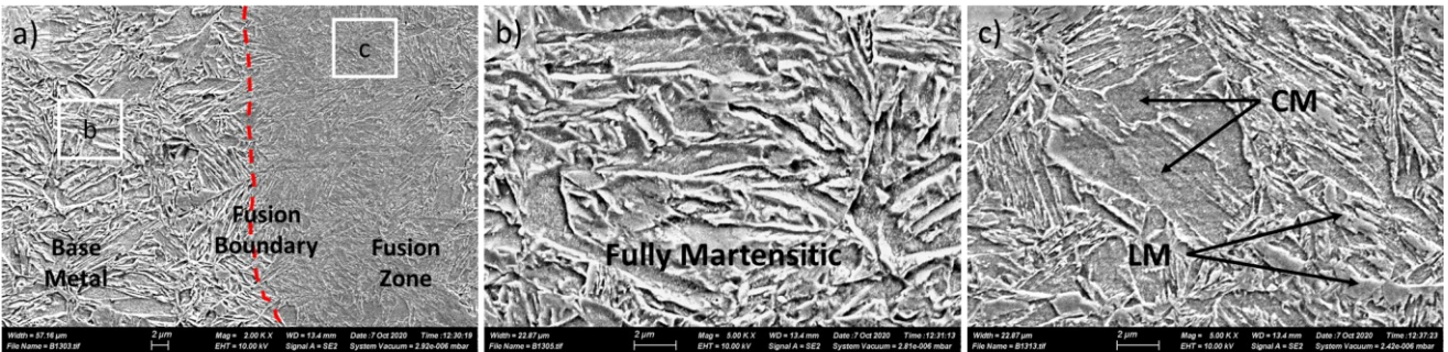
Figure 80: SEM images of the (a) fusion boundary of the WNHS condition at the location specified in Figure 79 as well as high magnification images of the (b) base metal showing a fully martensitic microstructure, and the (c) martensitic fusion zone showing a combination of prior martensite characterized by the darker concave morphology and fresh martensite characterized by the lighter convex morphology.
