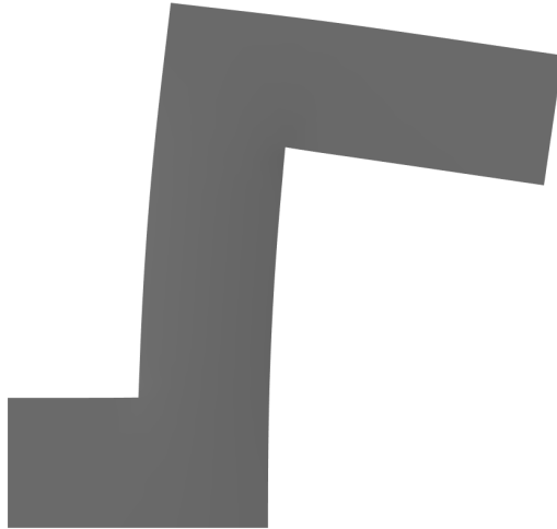
Figure 4.11: Sintering simulation output as a greyscale image for comparison with experimental data. One image is output for every simulated minute.
