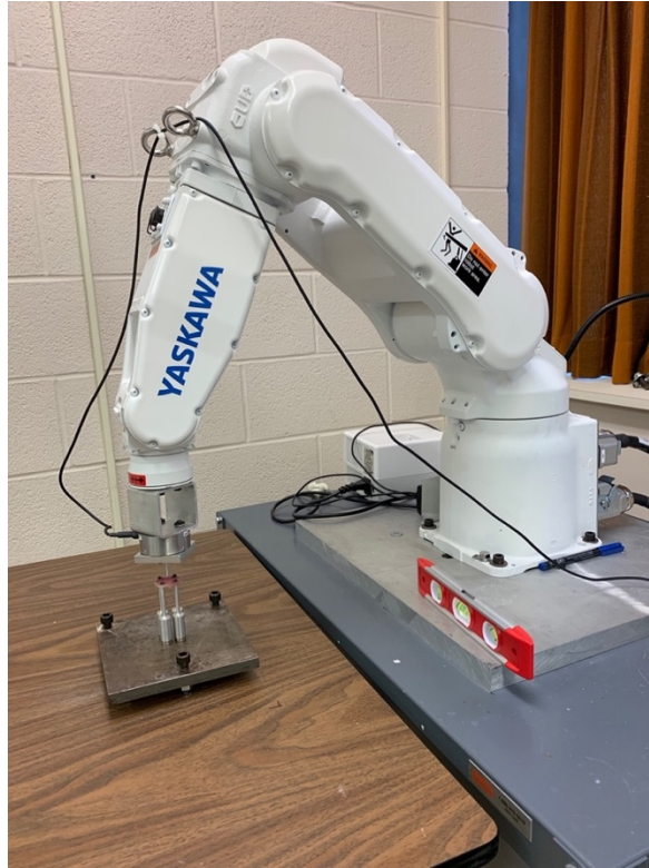
Figure 4.2.6. The microindentation setup, including the serial robot, load cell, aluminum stanchions, and carbon steel base.
