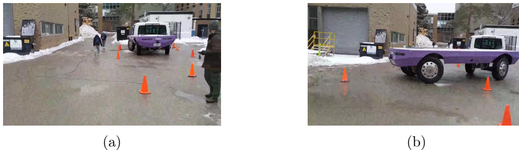
Figure 5.12: Displays the truck throughout an autonomous cornering maneuver performed experimentally. (a) Entering the corner. (b) Exiting the corner.
