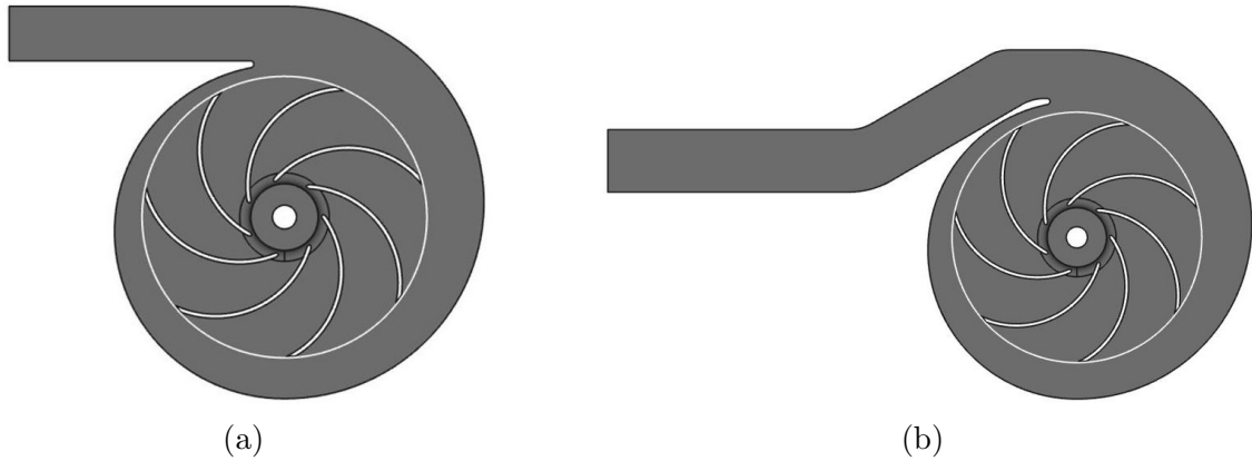
Figure 4.11: (a) Pump with tangential volute and (b) Pump with axial volute
