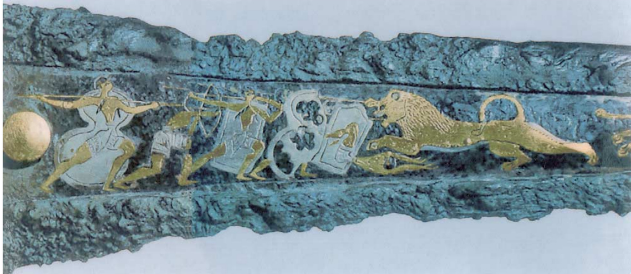
Figure 1.1: Cold-welded bronze dagger with intricate designs made of gold and silver pressed into it (reproduced with permission) [1].
