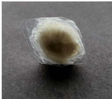
Fig. 2.59 Garment clasps. 3mm diameter earth magnets encased in milkweed silk fibers and thermally sealed with plastic lamination sheets.
