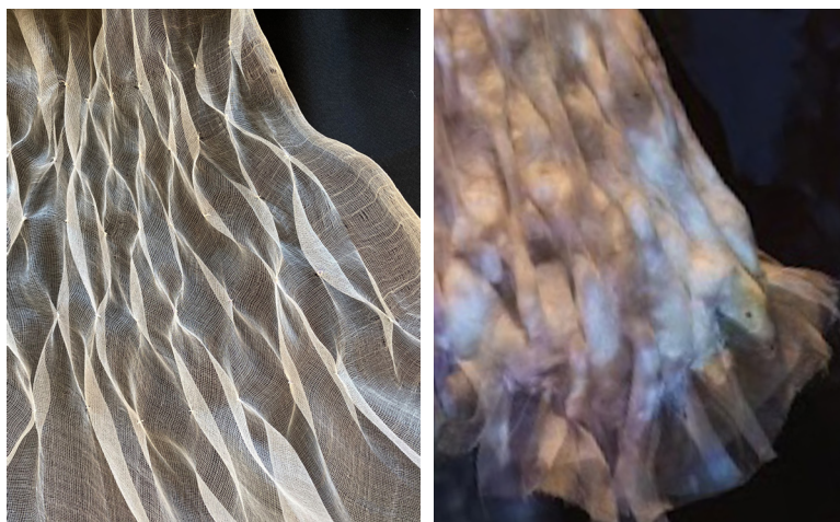
Fig. A.1 Blind tucks with honeycomb smocking before and after milkweed fibre infill.
