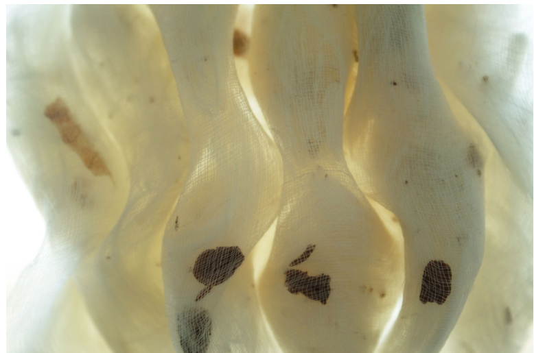
Fig. 2.36 Final material composite. Loose handwoven silk gauze, milkweed silk fibre infill, milkweed plant seeds, and silk thread.
