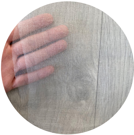
Fig. 2.14 Loose handwoven silk gauze as shell of the material composite.
