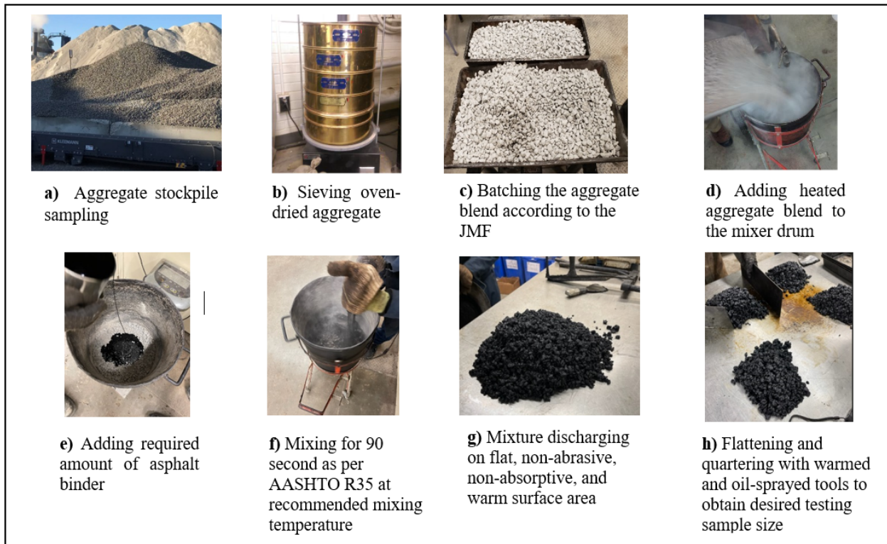
Figure 3-2: Laboratory Procedure for SMA and EME Asphalt Mixes Production in CPATT Laboratory
