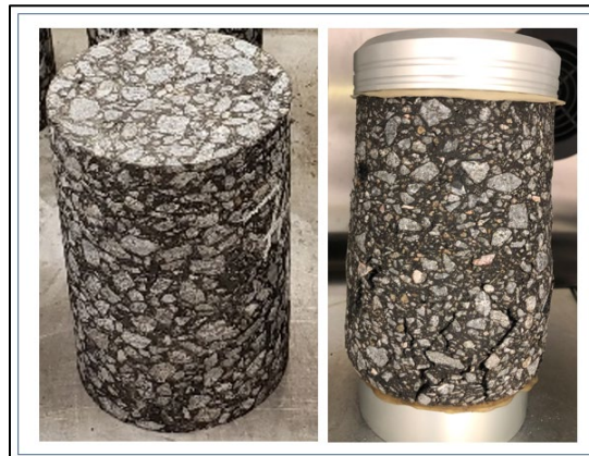
Figure 3-5: Flow Number Test Specimens Before (Left) and After (Right)
