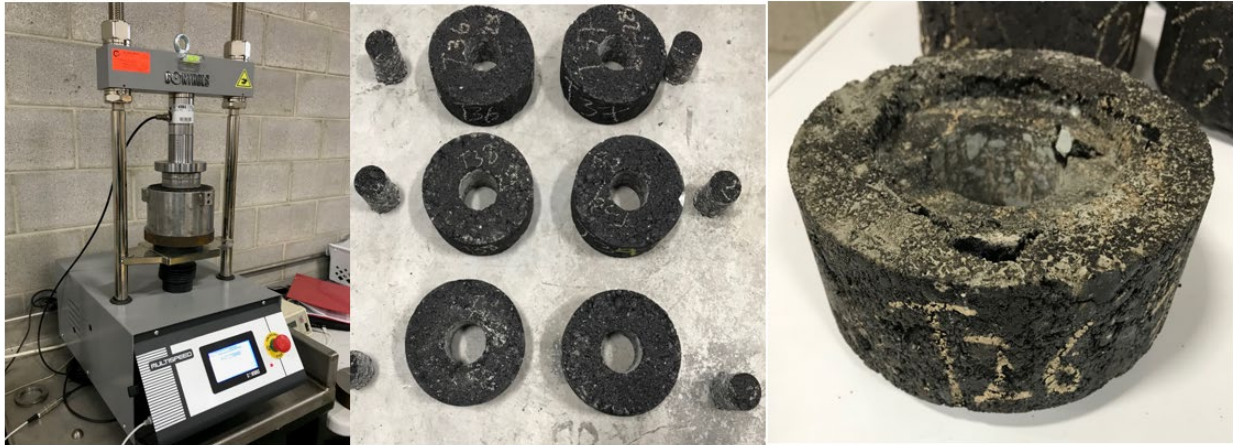
Figure 3-8: Uniaxial Shear Tester Monotonic Setup, and Test Specimens Before and After Testing
