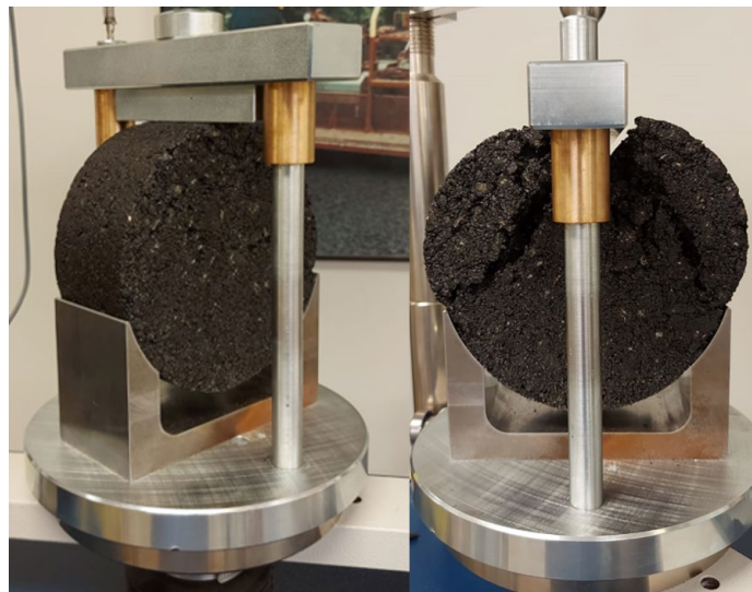
Figure 3-6: IDEAL-RT Test Fixture with Test Specimen Before (Left) and After Test (Right)
