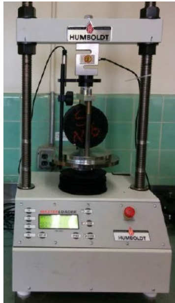
Figure 3-16: Indirect Tensile Strength Testing Equipment
