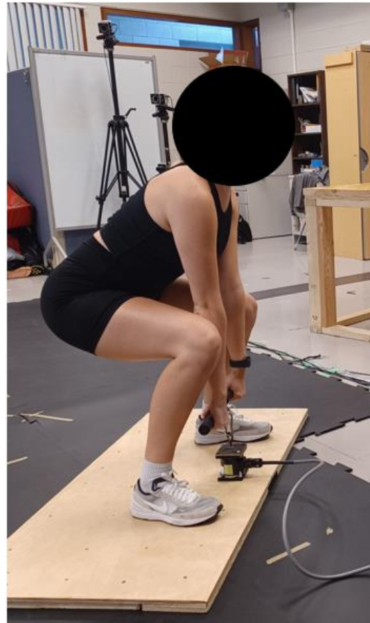
Figure 4-3: Maximal isometric lifting force protocol set-up. Participants were asked to maximally pull on the load cell in the vertical direction.
