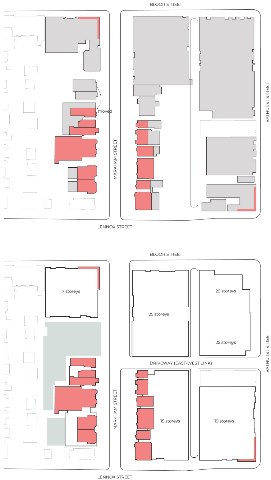
fig. 6.40 Site plan of Mirvish Village before work, grey signifying demolition (above) and proposed work (below)
