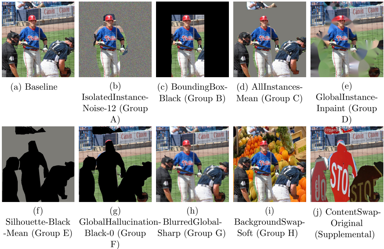
Figure 3.2: A representative subset of augmented images produced by our experiment modes. The experiment mode name is listed first, then the values after the ‘-’ represent mode details. Black/Mean/Noise are the color of the pixels used to replace any removed pixels. Numbers represent how many maximum pixels are added during the dilation operations (when applicable). Other adjectives describe experiment specific modes (e.g., sharp or soft for edge blurring). The group name in parenthesis refers to the relevant results in Table 3.1.
