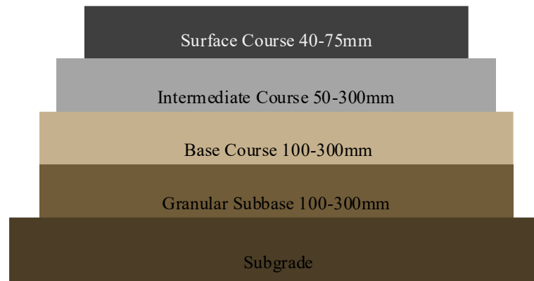
Figure 1-4 Typical structure of flexible pavement
