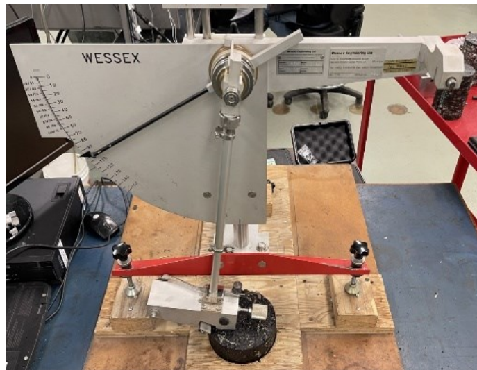
Figure 7-5 British Pendulum Skid Resistance at CPATT Lab
