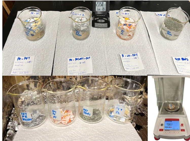
Figure 3-9 The water absorption test on an MPP plastic material at the CPATT lab
