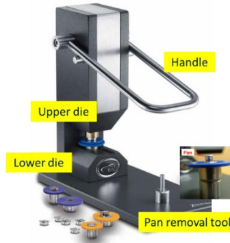
Figure 3-4 DSC encapsulation press
