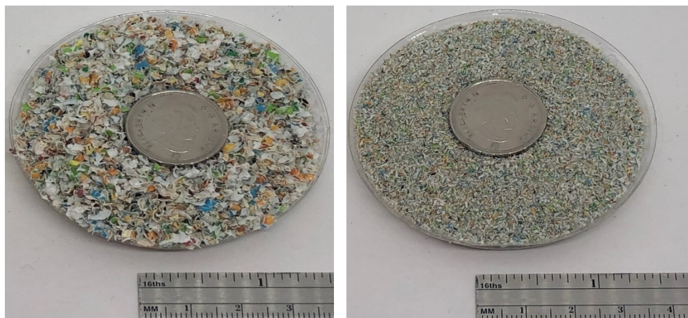
Figure 6-3 MPP in granule form (left) and powdered form (right)
