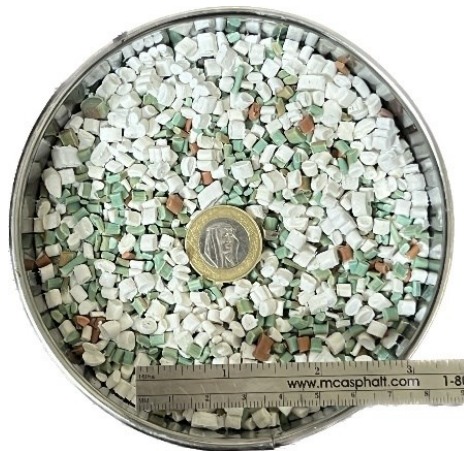
Figure 7-2 A picture showing the MPP pellets used in the asphalt mixture
