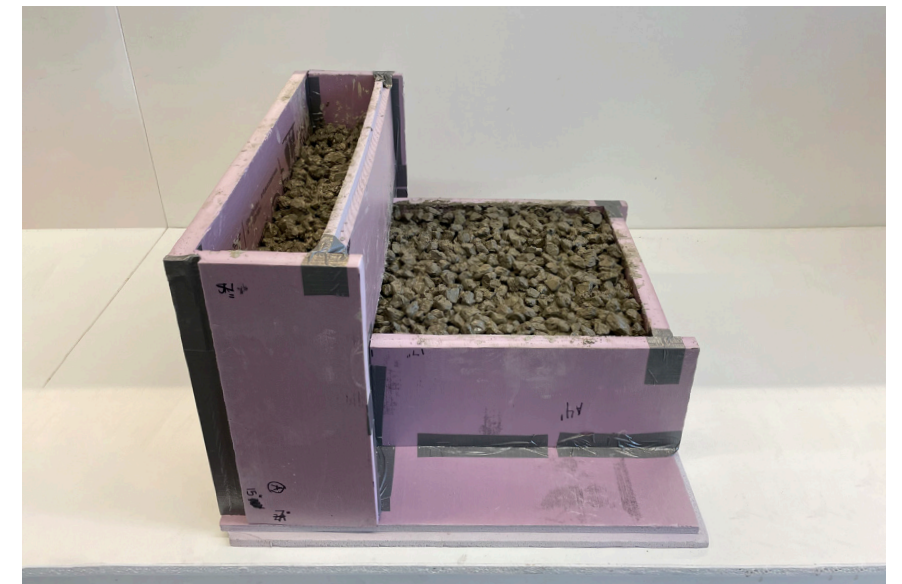
fig. 2.39 Complete pervious concrete cast in foam mould, January 2023.
