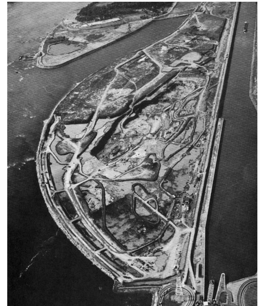
fig. 2.33 Aerial photograph of Notre-Dame Island showing the limestone quarry central to the island, formerly the island itself. Above Notre-Dame Island is the south end of the new Saint Helen's Island, where Swan Lake takes shape within the quarry that provided limestone for the site expansion, c. 1963-64.
