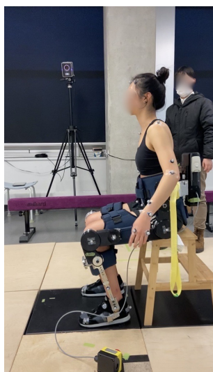
Figure 4.3: Force plate setup for STS trials without crutches.
