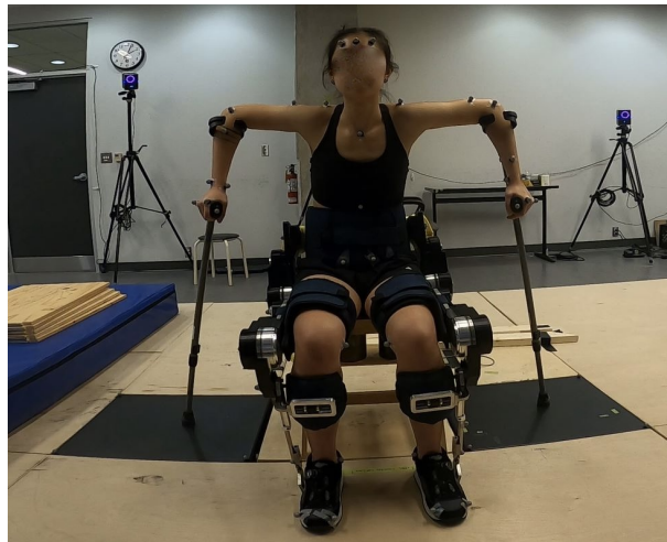
Figure 4.2: Force plate setup for STS trials with crutches.
