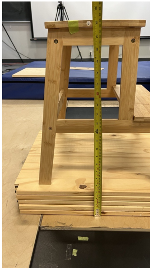
Figure 4.4: Five boards each with 2-cm thickness underneath the stool for STS trials performed at a higher seat height.
