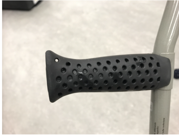
Figure 3.7: Sweat marks from a T member after the end of the exoskeleton session.
