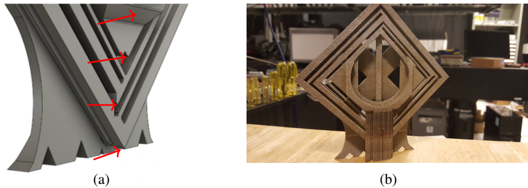
Figure 5.20: (a) Support attachment points for the TSK-45. (b) Supports shown on a prototype TSK-45.
