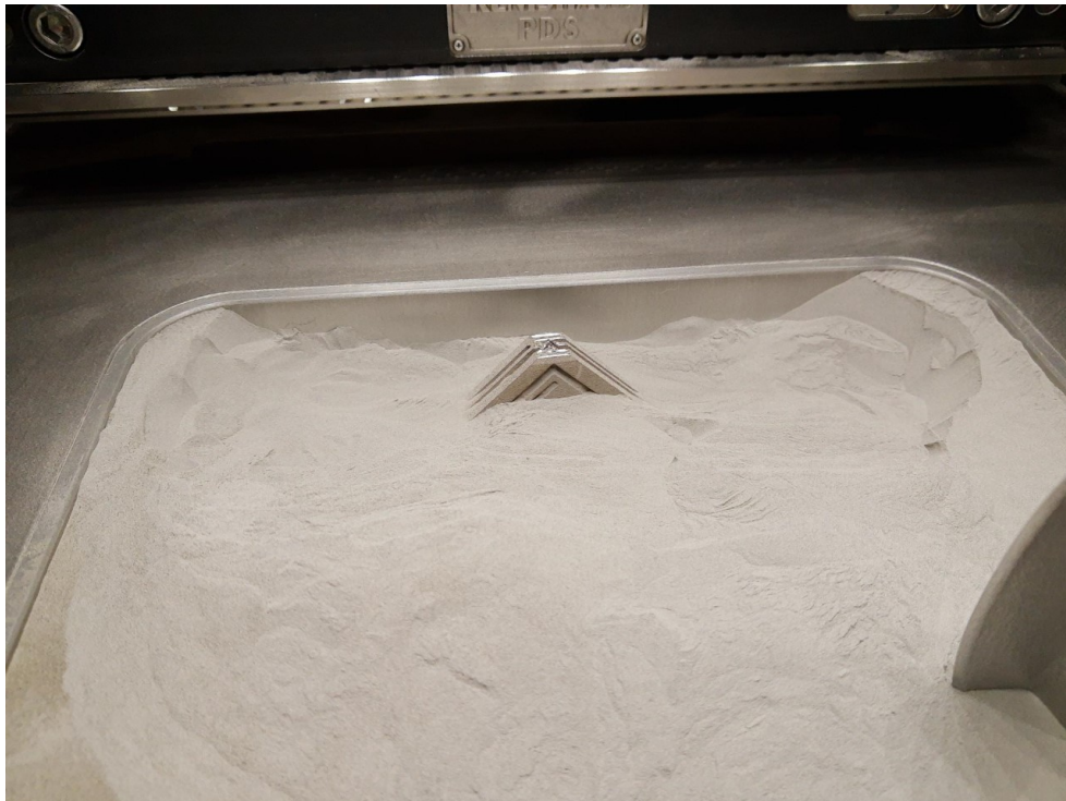
Figure 5.5: Completed structure in a sea of powder. This powder must be removed prior to use as it poses a health risk. Photo taken by Dr. Sagar Patel of the MSAM group.
