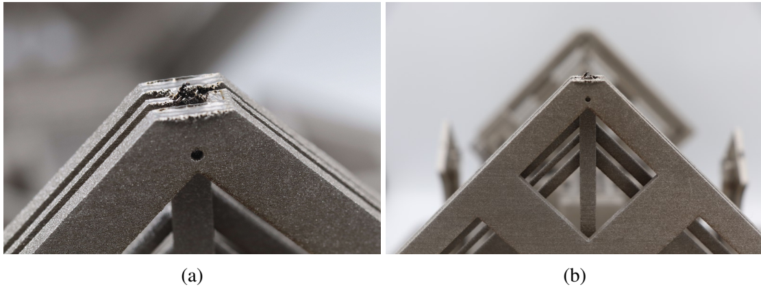
Figure 5.31: (a) and (b) TSK-45 incomplete on the final PORI build. The print failed with approximately 4 cm remaining. No further builds were attempted due to the project budget, timeline, and availability of the Renishaw AM 400.
