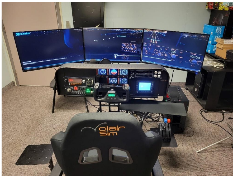
Figure 4: Medium-Fidelity Desktop Simulator Setup
