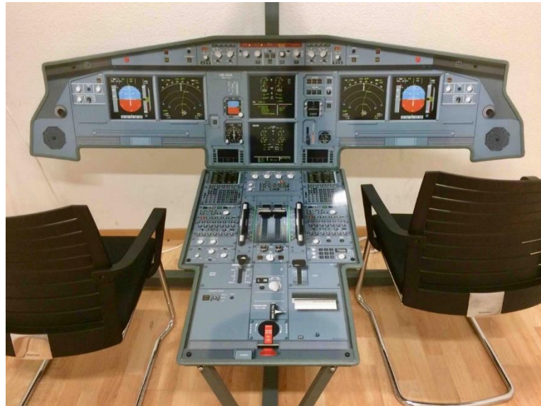
Figure 8: Paper Tiger Aircraft Model by Flight Vectors ( Cockpit Procedure Trainers - Paper Tigers - Cardboard Bombers, n.d. )
