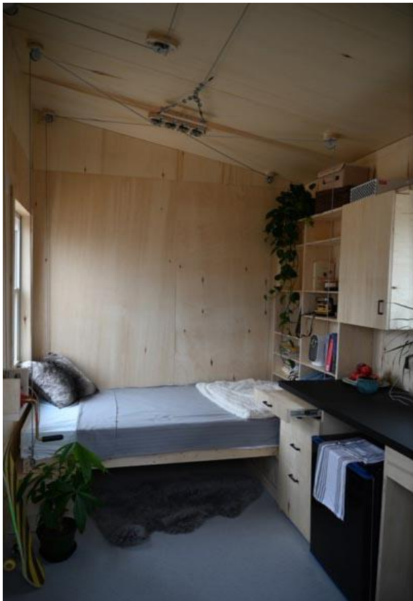
Fig. 32. The v1 interior, showing how the bed can be raised and lowered. (Photos by Leilei Zhao for the design-build studio and the Tiny Homes Research Project).
