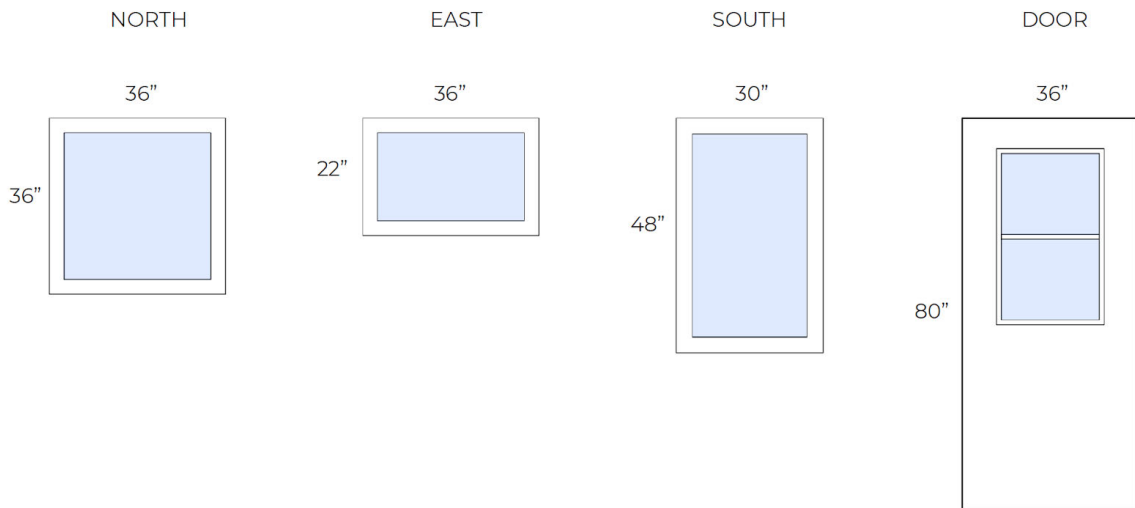
Fig. 108. The v1 window schedule, image from the Microhousing Design Studio Drawing Set (Chen and others 2021).
