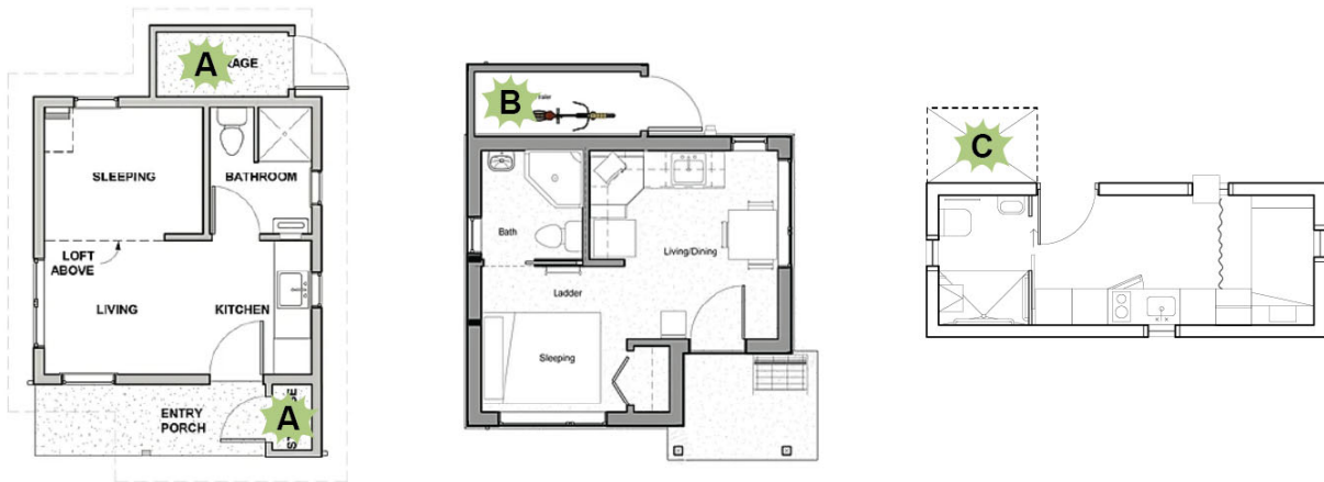
Fig. 117. Green stars mark the outdoor storage at two Emerald Village homes, and a planned location for v2. (Image by author, using drawings by Nir Pearlson Architect and Dustrud Architect, retrieved from https://www.squareonevillages.org/design ).
