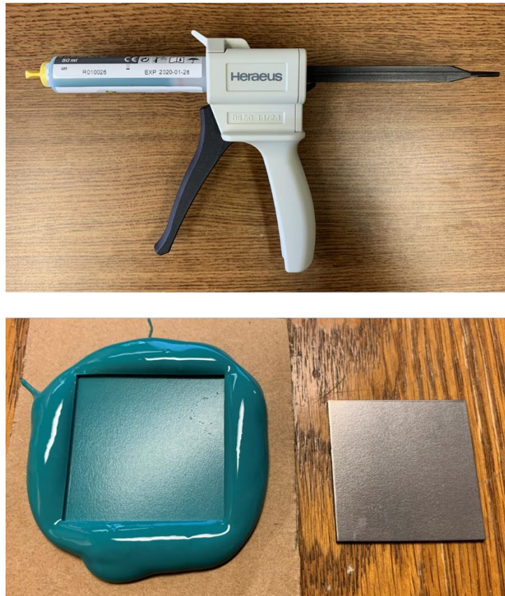
Figure 4-11: Surface replication apparatus, Top: Application gun, Bottom: 1509m Mid sample and its replicate.
