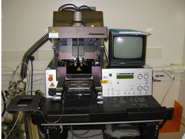
Figure 3.6: Image of the SUSS MA6 mask aligner present in the G2N lab
