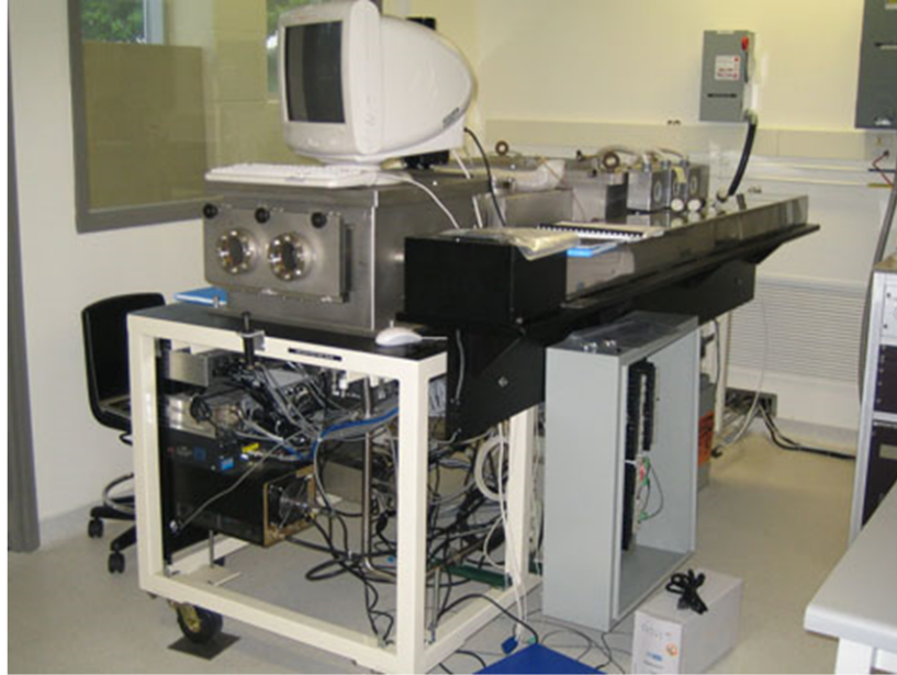
Figure 3.5: Image of the WLOS cluster sputtering system in the G2N lab used in this work
