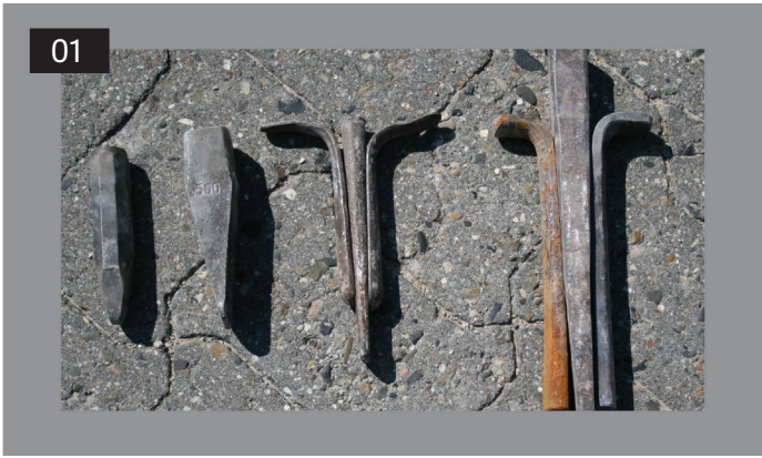
Fig. 1.10 Photograph showing plugs and feathers in various sizes, Reiner Flassig, Wikimedia Commons.
