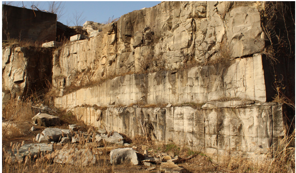
Fig. 2.13 Queenston Quarry, showing the change in lithology at the exposed surface, image by author.
