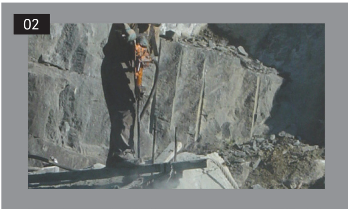
Fig. 1.11 Photograph showing worker using Jackhammer drill in a quarry, Halvard, Wikimedia Commons.
