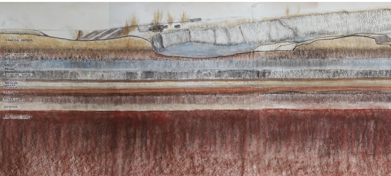
Fig. 1.5 Perspective Section Facing West Side of Queenston Quarry, 22" x 90", at 1:500 scale, graphite and pencil drawing by author. This geological section shows the depth of quarrying activities once present on the landscape. The volume of geological formation removed from site is revealed, along with the different formation layers beneath the Queenston Quarry. It also shows the gasport member exposed on the west side of the quarry.
