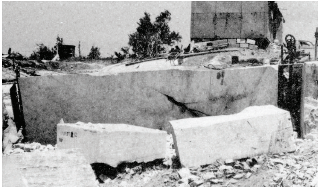
Fig. 1.19 Mill blocks of marble cut by wire saw at Tatlock quarry of Omega Marble Tile and Terrazzo Limited., D.F Hewitt, Building Stones of Ontario , Part 1, Introduction, 38.
