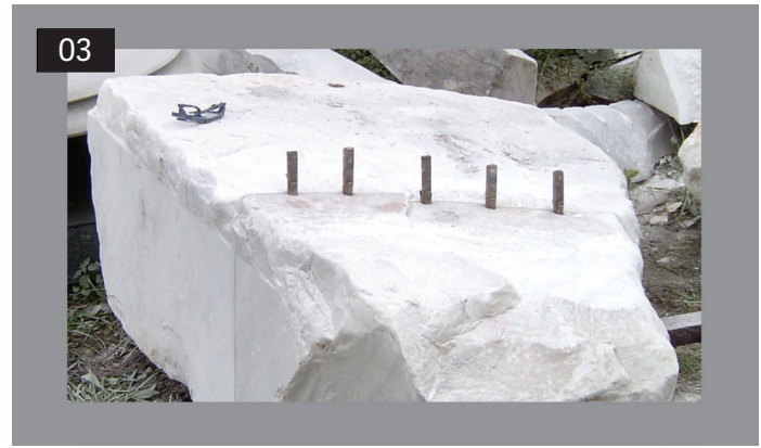
Fig. 1.12 A block of marble prepared with wedges for splitting, Reiner Flassig, Wikimedia Commons.
