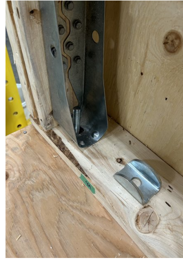
c) Left side hold down (easy to remove nut and curved washer)
