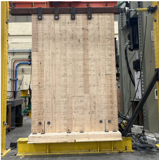
a) Modified CLT setup (note additional pivot point between actuator and column, HSS shifted to account for pivot)
