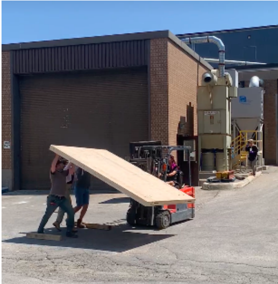
a) Drop Test #1 Starting Position
