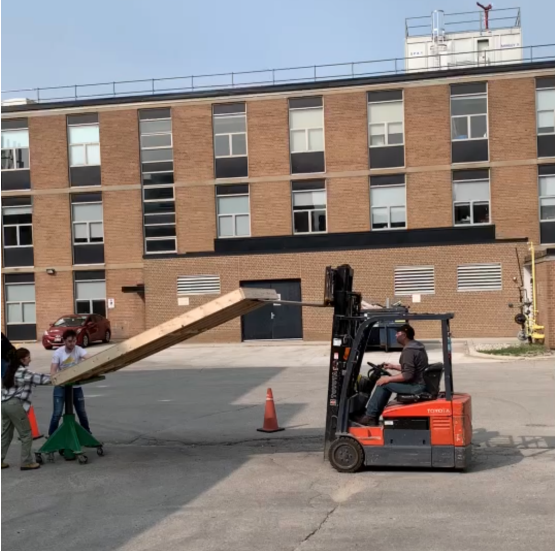
a) Drop Test #1 Starting Position
