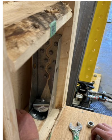
d) Right side hold down (tight to unscrew, curved washer difficult to remove – jammed in hold down)
