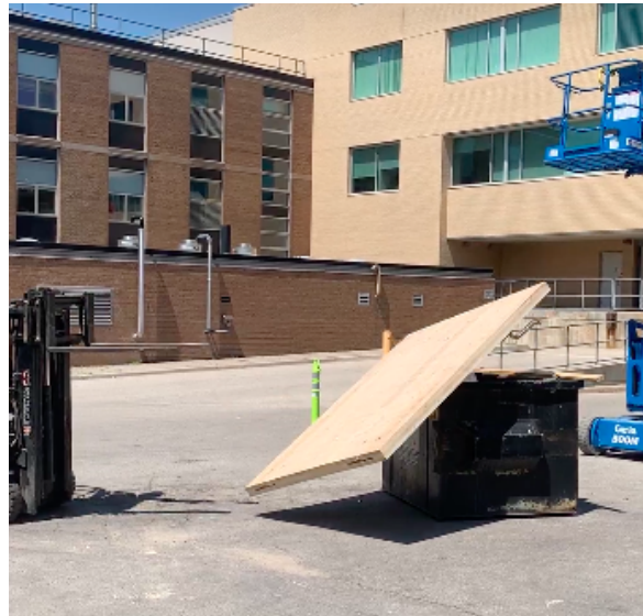
d) Drop Test #2 Mid-Drop
