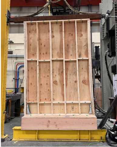
a) Overall deformed panel (before retracting actuator to 0 mm disp.)
