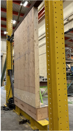
a) Back of panel (note the sheathing layout)
