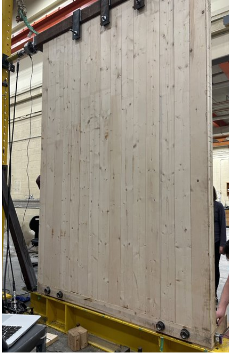
a) Back of panel (no visible damage)
