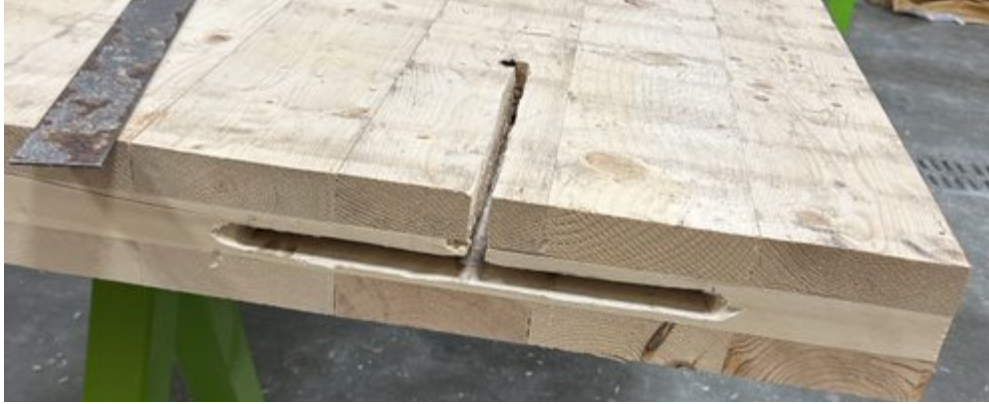
a) Right side connection slot in panel
