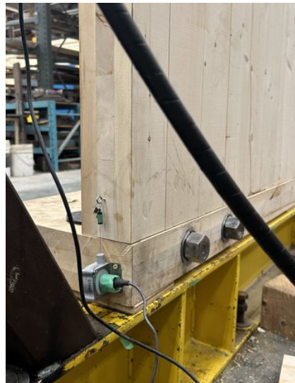
d) Right side connection (rear view; no visible damage)
