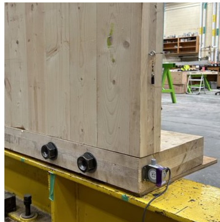
c) Left side connection (incl. back bolts through base)
