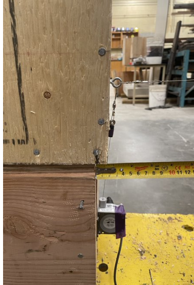
b) Offset between panel and base (~1.5-2 cm)
