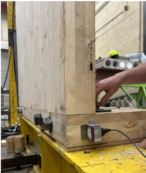
c) Left side connection (no visible damage)
