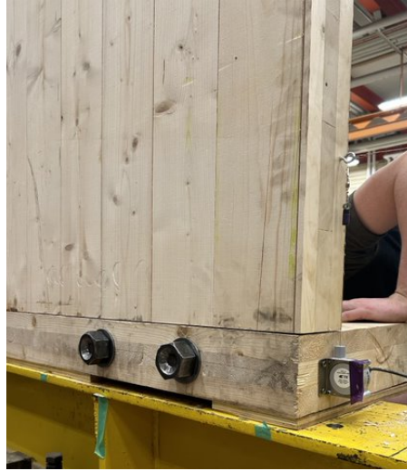
b) Left side connection (rear view; no visible damage)
