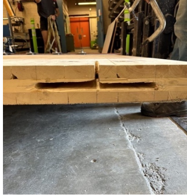
b) Right side connection slot (no visible damage)
