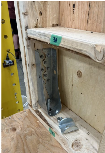
c) Left side hold down (easily unscrewed and washer easily removed)
