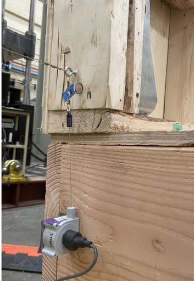
a) Left side hold down (panel sliding off of base)
