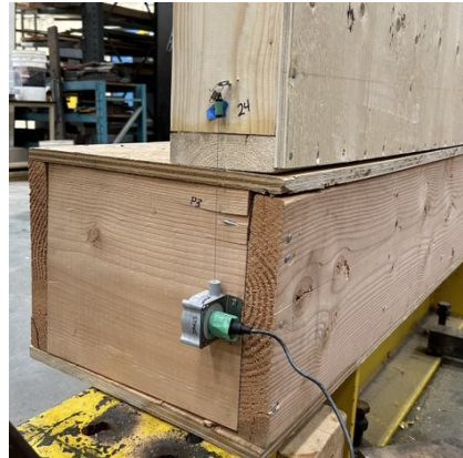
h) Right side hold down (back; no visible damage on bottom plate other than mark on top right)
