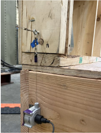
a) Left side hold down (bottom plate end grain)
