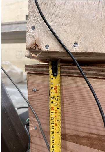
e) Right side hold down uplift (back)
