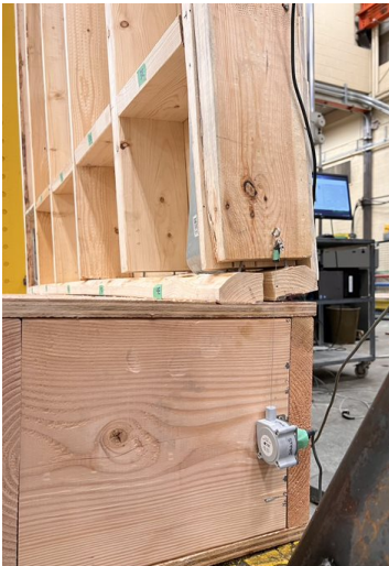
d) Right side hold down uplift and cracking (4E)
