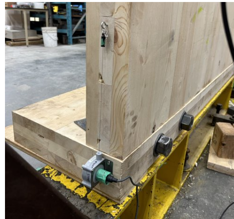
e) Right side connection (incl. back bolts through base)
