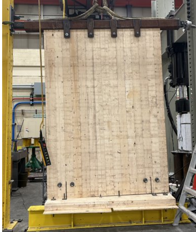
Figure 5.3 – Final Displaced Shape of CLT #1 After Phase 1
