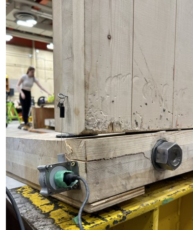
c) Right side connection uplift (note base crack that extends from bolt)
