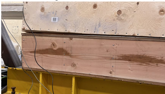
g) Right side hold down (near 4E) uplift (back)
