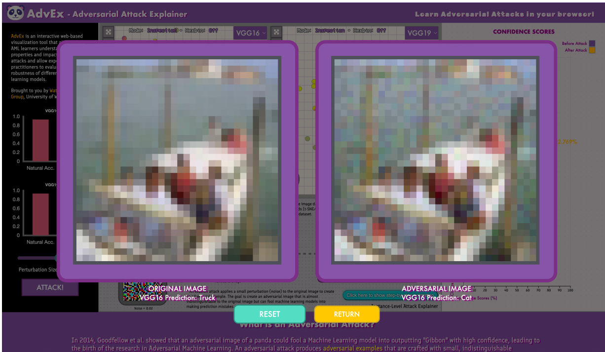
Figure 4.6: By clicking on the image thumbnails in the attack explainer, the user can view an individual image in an enlarged format or enter comparison mode, which displays the original and adversarial images side by side. This way, the user can identify the subtle perturbations applied to create the adversarial image.
