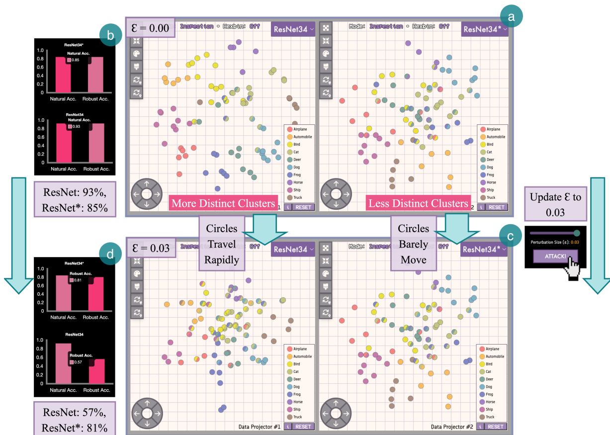
Figure 7.1: An AI expert using ADVEX to investigate ResNet models trained naturally & adversarially under the FGSM attack. Here, she increases \epsilon from 0.00 to 0.03 and observes the changes in the two models' embedding distributions and prediction accuracy.
