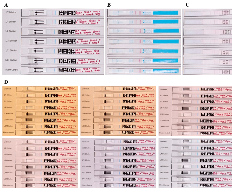
Figure 4.1 - Overview of serially diluted LFA tests under controlled light conditions. Representative images of the three commercially available (A: Quidel Strep A, B: ICON DS Strep A, C: BD Veritor Flu A+B) LFAs performed in serial half dilutions from 1/2 to 1/64 using the provided positive control reagent under 5500K light. D: Representative images of the controlled lighting conditions that each assay and dilution series were collected under (The Quidel test is shown as example). Lighting conditions started at 3200K (upper left image: warm – orange tint) and underwent twenty-four 100K increments to 5500K (bottom right image: cold – blue tint).
