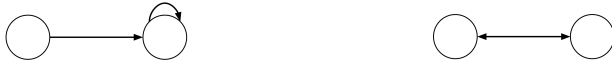
Fig. 1: Multiple instances of a transition system for the constraint: every state must reach a state that is reachable from itself.
