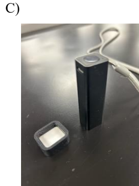
Figure #8: Illustration of A) Pico scanner schematic and usage diagram and B) scanner with calibration cap on and C) off, with D) usage of the device demonstrated.
