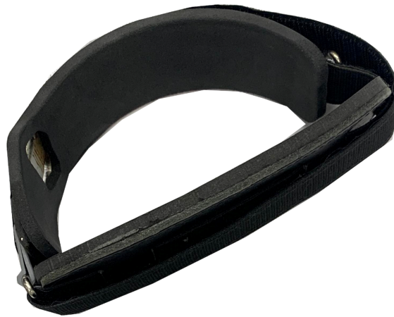
Figure 3.2: H3 Exoskeleton generic interface with aluminum backing and EVA foam compliant surface.
