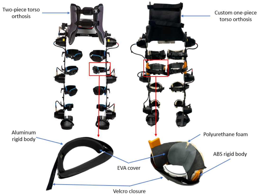
Figure 4.2: Generic (left) and custom (right) surfaces mounted to the H3 exoskeleton. The two piece generic torso orthosis has a much lower surface area compared to the one-piece custom orthosis. The custom limb surfaces are layered thicker than the generic interfaces, and have a larger circumferential surface area length.
