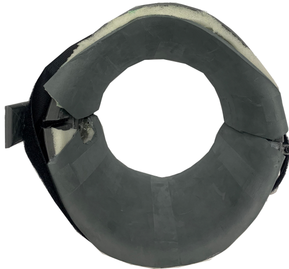
Figure 3.3: Top down view of the H3 Exoskeleton custom surfaces manufactured from PLA
