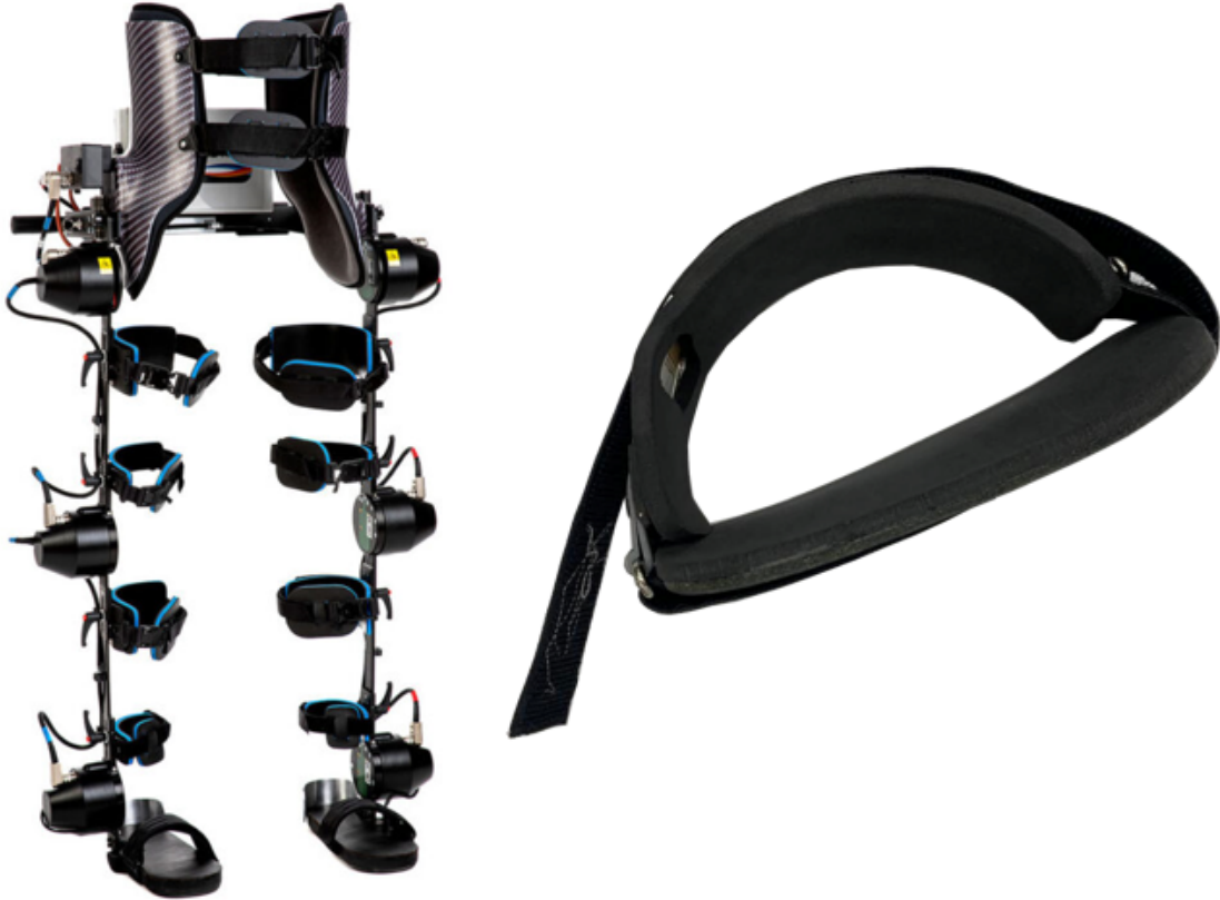
Figure 8.3: The H3 exoskeleton and one of the coupling interfaces. The coupling interfaces are “generic” by design, intended to fit a wide range of individuals and as such are not perfectly circular, nor half of the circumference of a circle to allow for ease of use.
