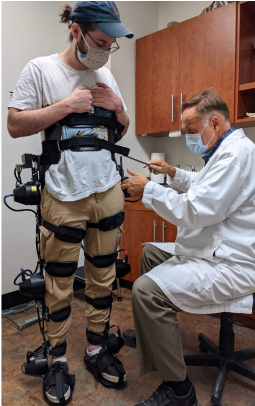
Figure 3.6: Photo of Al Moore - right (OBS) working with Christian Mele - left on fabricating and measuring out a Torso Orthosis for the H3 Exoskeleton.
