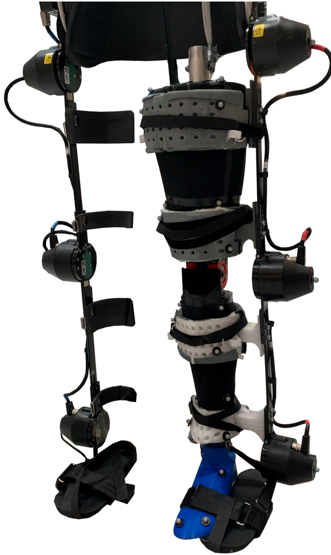
Figure 3.4: H3 Exoskeleton suspended with 2-DoF mannequin on the stationary testbench. The exoskeleton is mounted with the custom surfaces, and VICON markers are placed along the exterior to capture kinematic information.
