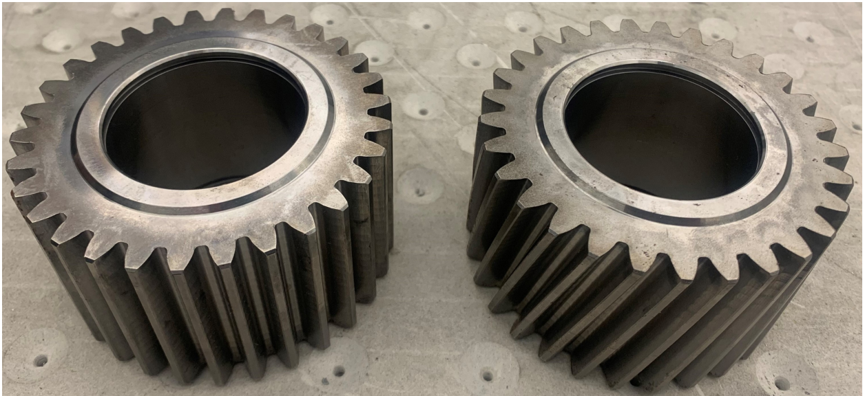
Figure 5.2: Finished workpiece for spur(left) and helical (right) case studies
