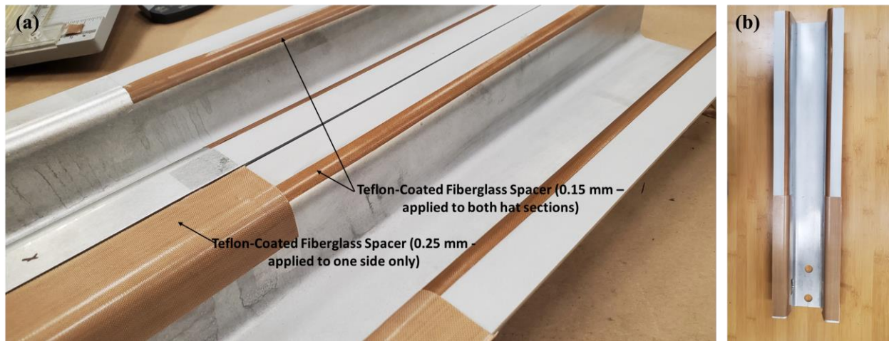
Figure 62: (a) Teflon-coated spacers to maintain bond line thickness and reduce edge effects and adhesive spew, (b) Hat section ready for adhesive or hybrid joining application.
