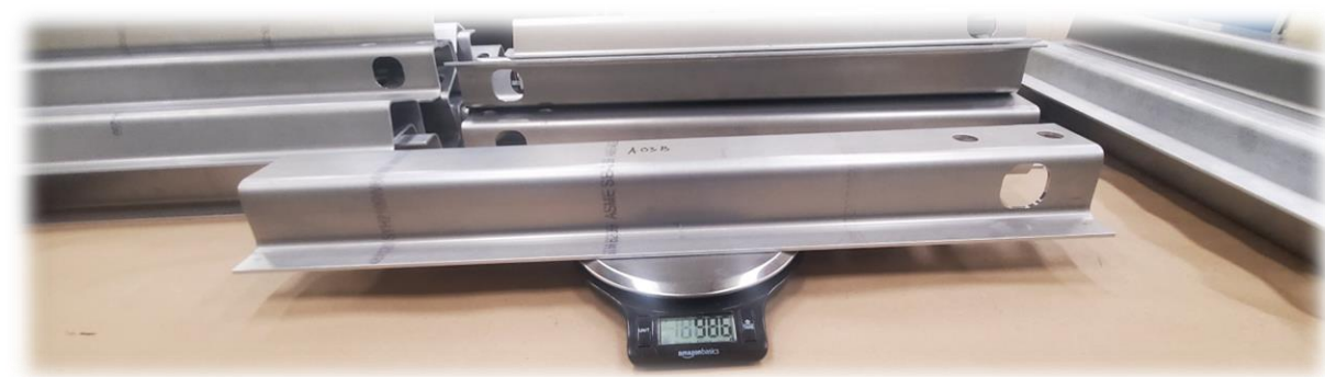
Figure 59: The weight measurements of the hat section to ensure weight precision.
