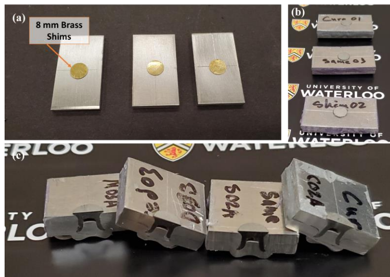
Figure 55: (a) 0.17 mm thick brass shims (8 mm diameter) applied to the centre of the joining area, (b) Specimens prepared using variations of the traditional hybrid joining technique, and (c) cross-sectioned specimens.
