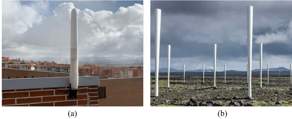
Figure 1.2: (a) Bladeless wind turbine and (b) bladeless wind farm [163].
