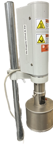
Viscometer setup during measurement with inner cylinder (bob) and outer cylinder covered by solution container
