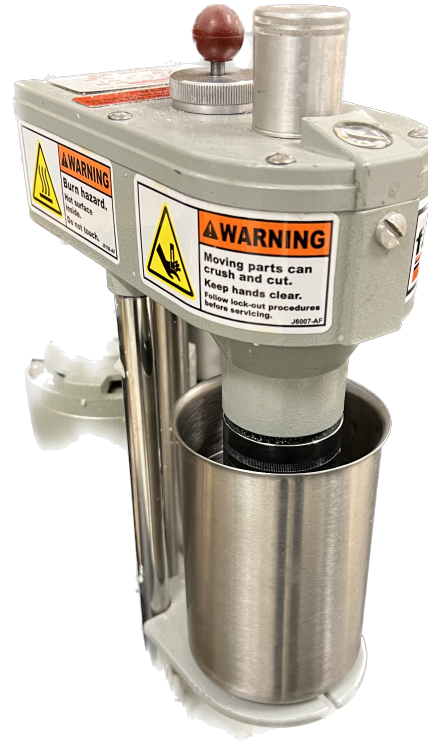
Viscometer setup during measurement with inner cylinder (bob) and outer cylinder covered by solution container
