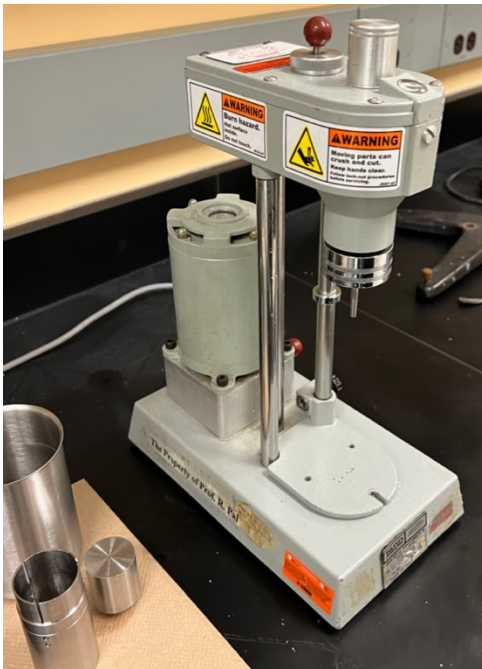
Viscometer setup before measurement with inner cylinder (bob) and outer cylinder displayed
