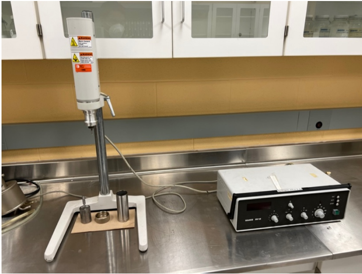
Viscometer setup before measurement with inner cylinder (bob, left) and control panel w/ digital display (right)
