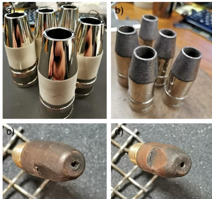
Figure 2-8 Photo of a) uncoated and b) coated RSW copper electrodes; and the c) uncoated and d) coated electrodes that undergo multiple welding, adapted from [76]
