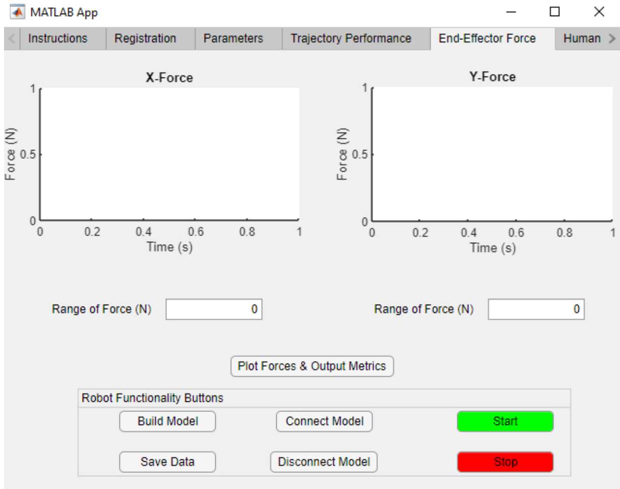
Figure A.10: Force performance tab, which shows the time series of the 2D force exerted by the patient on the end-effector and the corresponding range of forces.
