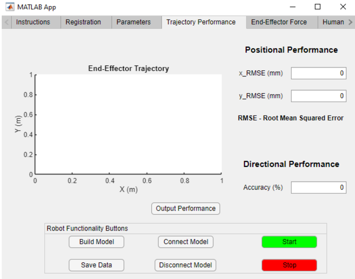
Figure A.9: Trajectory performance tab, which shows both the positional and directional performance of the user during their trial.
