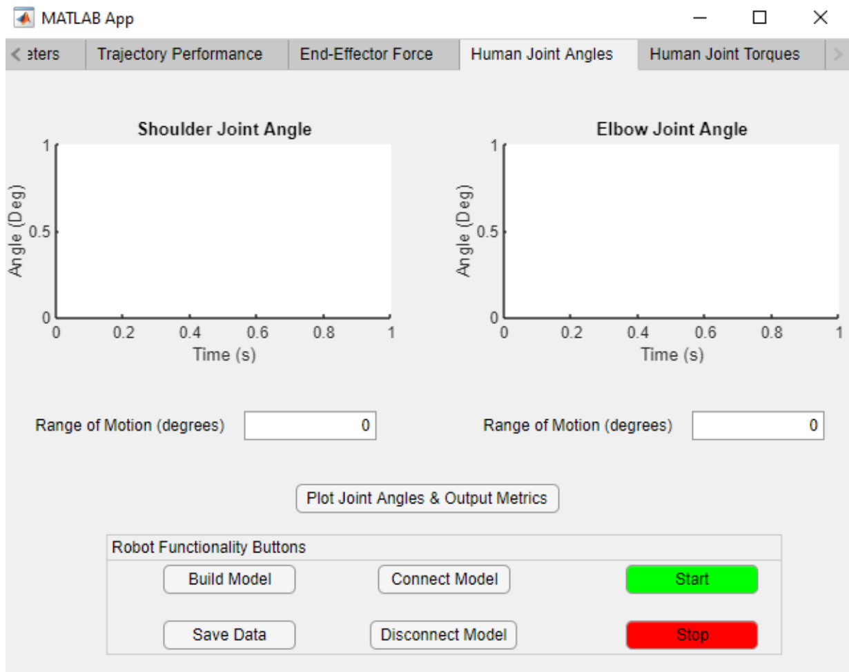
Figure A.4: Human joint angles tab, which shows the time series of the joint angles and the corresponding range of motion.
