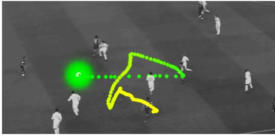
Figure 33: Model simulation for unbiased attention during ball tracking: Tracking of an unpredictable ball-passing sequence; ball trajectory shown in yellow (earlier position) to green (later position) gradient; attention distribution in green is normally distributed about ball motion.
