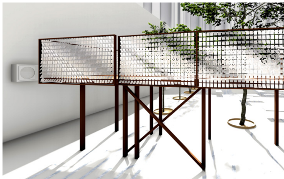
Fig. 6.25 Example of Kinetic Facade
