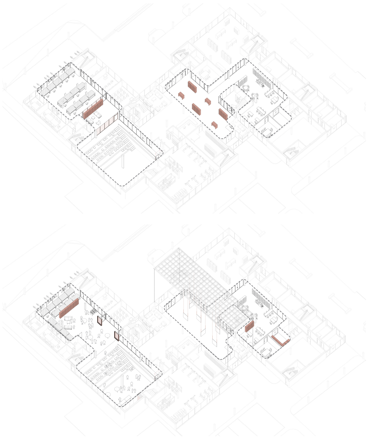
Fig. 4.26 Flexible usage of folding walls and movable furniture. The structural beam system of the gallery space lends itself to suspended exhibitions.
