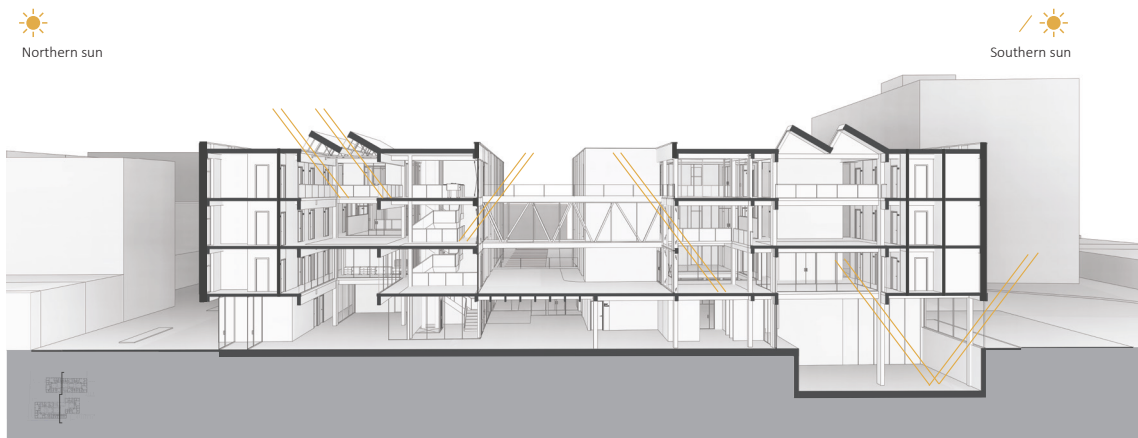
Fig. 4.38 Voids within the building help the dissemination of diffused light. While light wells bring in east and west sunlight, glass facades and skylights help bring in south and north lighting making the all-day daylighting possible.
