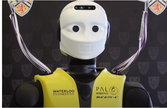
Figure 3.1: REEM-C Humanoid Robot, with RGB-D camera shown on forehead
