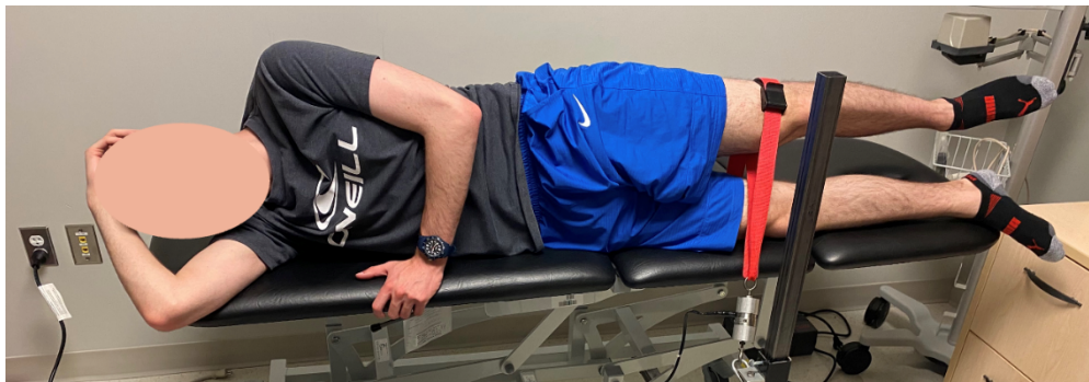
Figure 16: Participant Positioning during the Contracted State Trials – Participants laid on their right side. During the SWE measurements, they performed an external rotation and extension of their left hip, while keeping their leg straight to activate the gluteus maximus. This pulled on the force transducer and updated the force that the participant was exerting on the biofeedback system set-up in front of them.
