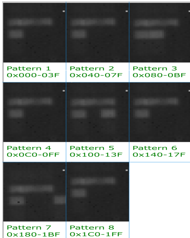
Figure 5.16: Photon emission pattern in B_1 , showcasing periodicity as addresses repeat every 0x200 bytes.
