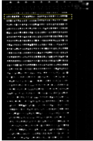
Figure 4.10: Photon emission from SRAM holding 0x4A in the target word, showcasing the selected area of interest.
