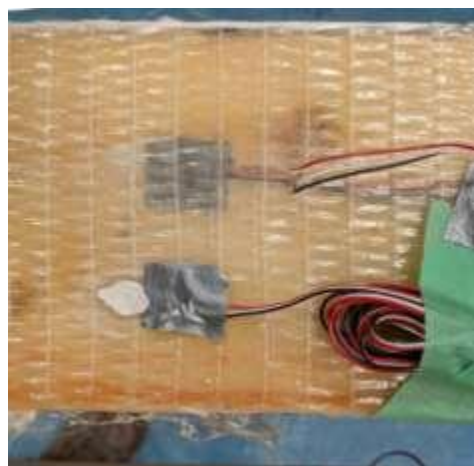
Figure 3.4: Strain gauge installation on GFRP laminates
