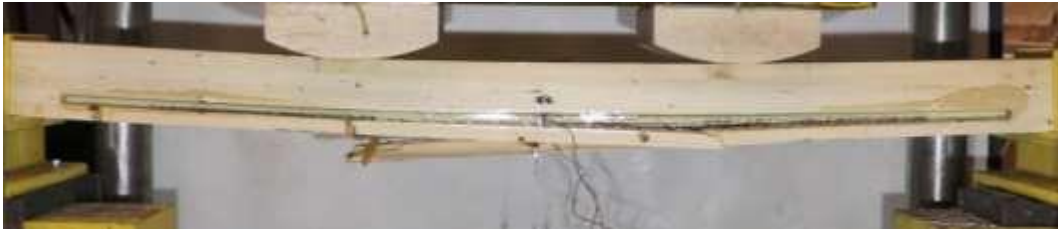
(b) Initial failure
