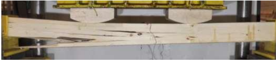
(b) Initial failure
