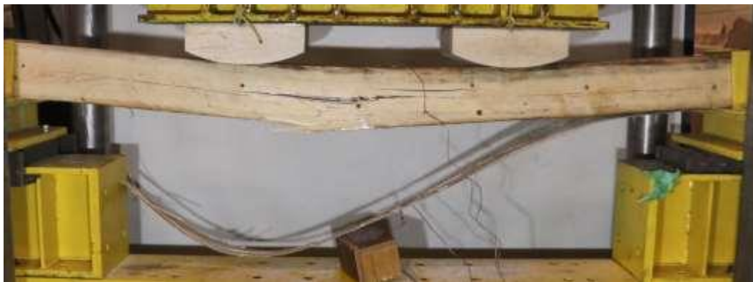
(b) Initial failure, FRP debonding
