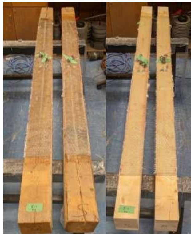
(d) Cured GFRP laminates on sawn timber (left) and glulam (right)
