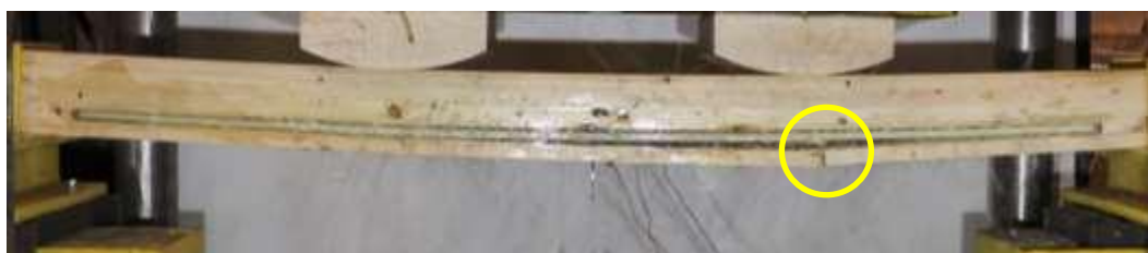
(b) Initial failure
