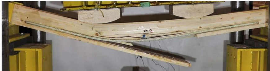
(d) Overall beam at ultimate failure
