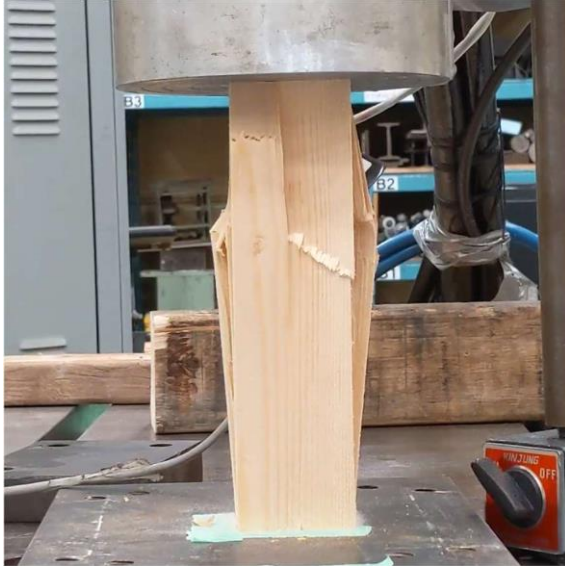
(a) Ultimate failure
