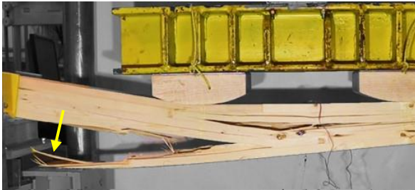
(c) Failure at FRP termination point in GF-2
