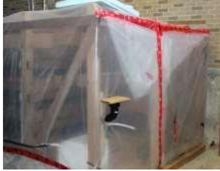
(a) Humidity chamber*
