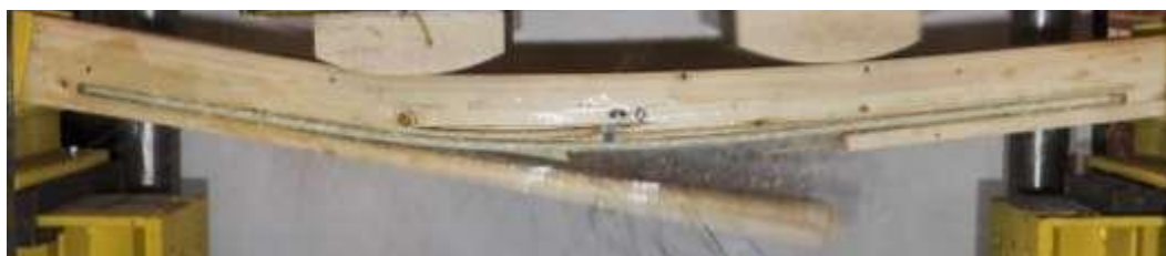
(c) FRP resin failure
