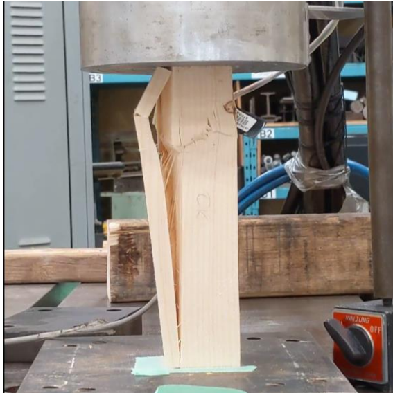
(a) Ultimate failure
