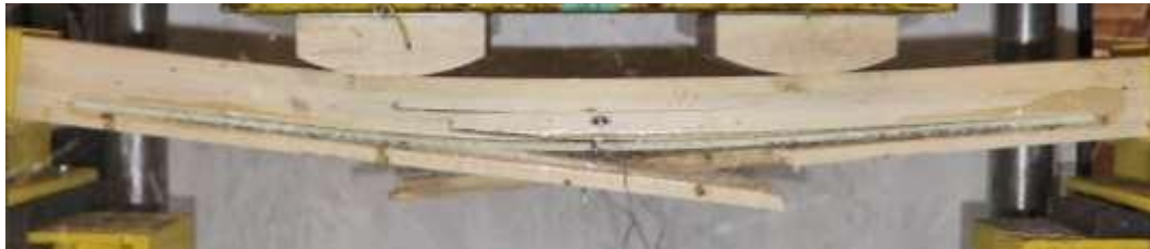
(c) FRP resin failure
