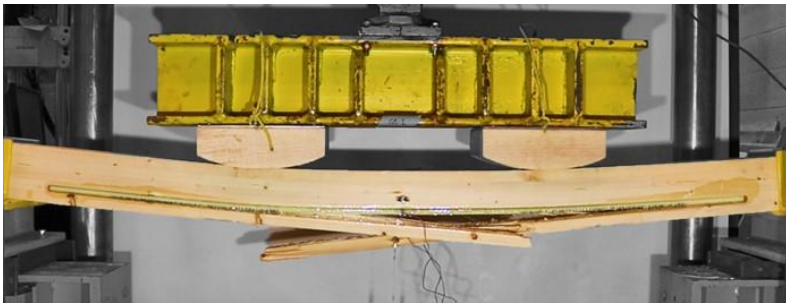
(3) Wood-cover failure; secondary peak loading
