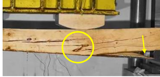
(b) Failure at FRP termination point in SF-2
