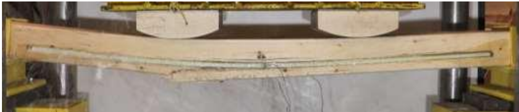
(c) FRP resin failure
