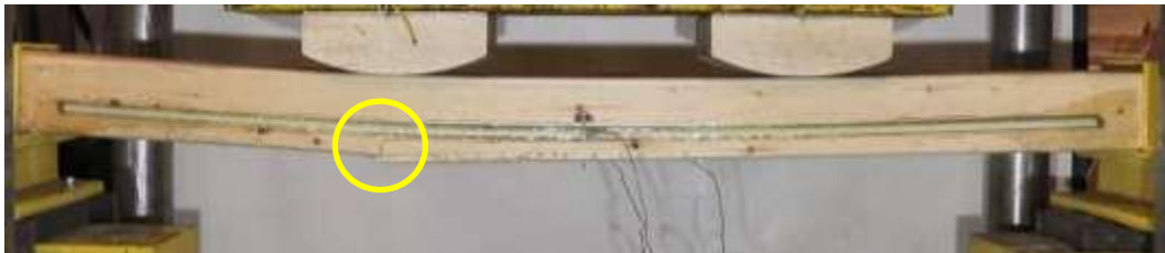
(b) Initial wood failure; string pot disconnected
