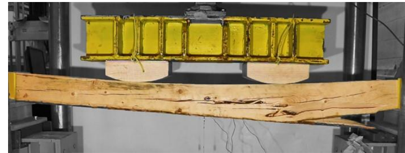
(4) Crack progresses through pre-existing surface checks
