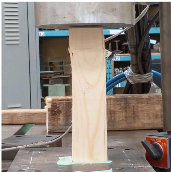
(a) Ultimate failure
