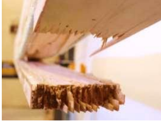
Figure 4.23: Ruptured finger joint in GB-1
