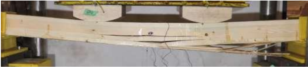
(b) Initial failure
