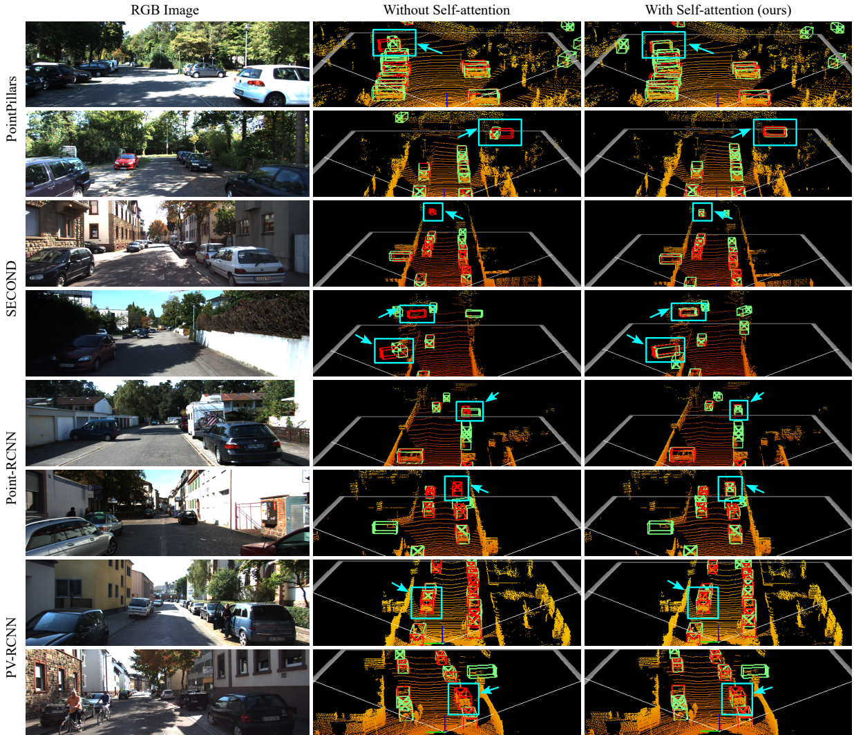
Figure 4.8: Qualitative comparisons of our proposed approach with the baseline on the KITTI validation set. Red represents Ground-Truth bounding box while Green represents detector outputs. From left to right: RGB images of scenes; Baseline performance across state-of-the-art detectors PointPillars [83], SECOND [184], Point-RCNN [144] and PV-RCNN [143]; Performance of proposed FSA module-augmented detectors. Viewed best when enlarged.
