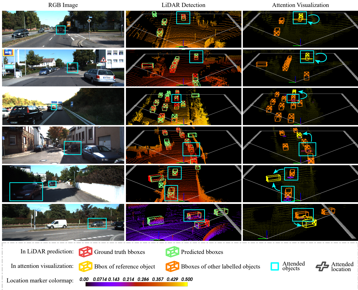
Figure 4.9: Visualization of attention maps produced by our proposed FSA-variant on SECOND [184] backbone. We analyze the implications of the produced attention maps in Sec. 4.5.5.
