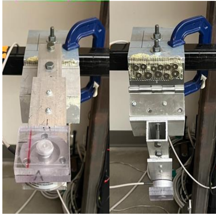
Figure 8: Load Cell Setup for Experiment 2
