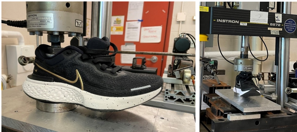
Figure 3.2: Exemplar Men's ZMX shoe undergoing stiffness quantification via the materials testing system.
