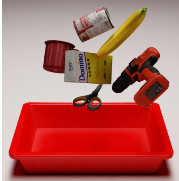
Figure 3.2: Physics-based data synthesis: Items are dropped into the photorealistic, physics-driven metaverse digital twin of different manufacturing scenarios.
