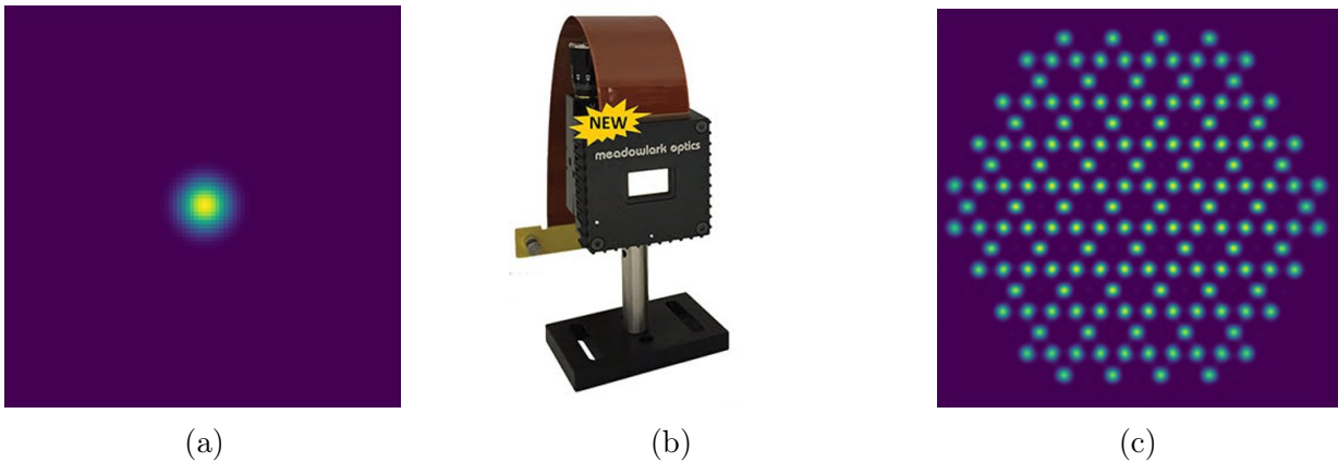
Figure 2.2: Generating arbitrary geometry of optical tweezers with diffractive optical elements.
